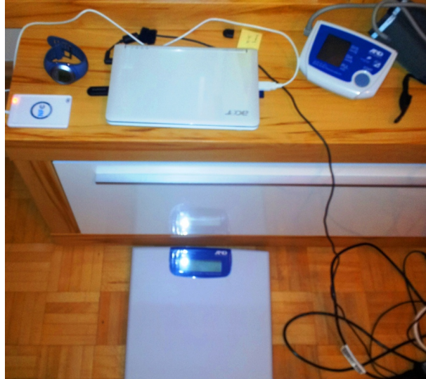
Figure 3.2. Patient environment consisting of a data hub (netbook), smart card reader, blood pressure meter, weight scale and sports watch
