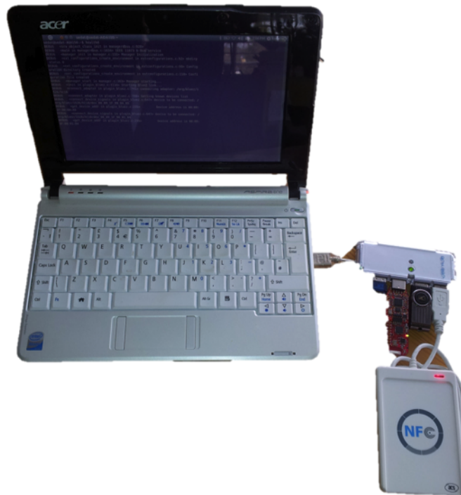
Figure 2.17. The Acer Aspire One was used as an AHD with Bluetooth, ZigBee, ANT+ dongle and NFC card reader
