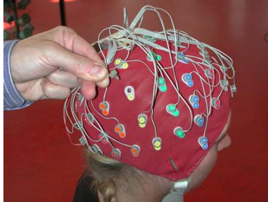
Figure 4.2: A 64 channel BIOSEMI headcap was used together with active electrodes to record AEPs. Figure from http://www.biosemi.com/pics/apply_cap3_large.jpg .
