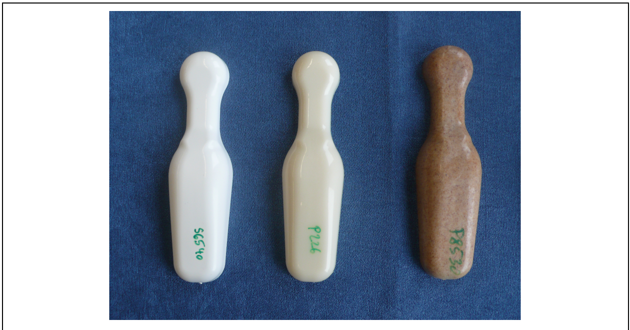
Figure 8-5: (from left to right) BioFlex S6540, P226, and Fibrolon P8530
