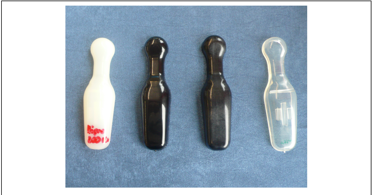
Figure 8-4: (from left to right) Hiprolon 200 VN, EcoPaxx Q 150D, EcoPaxx Q-X70208, BioGrade C7500,
