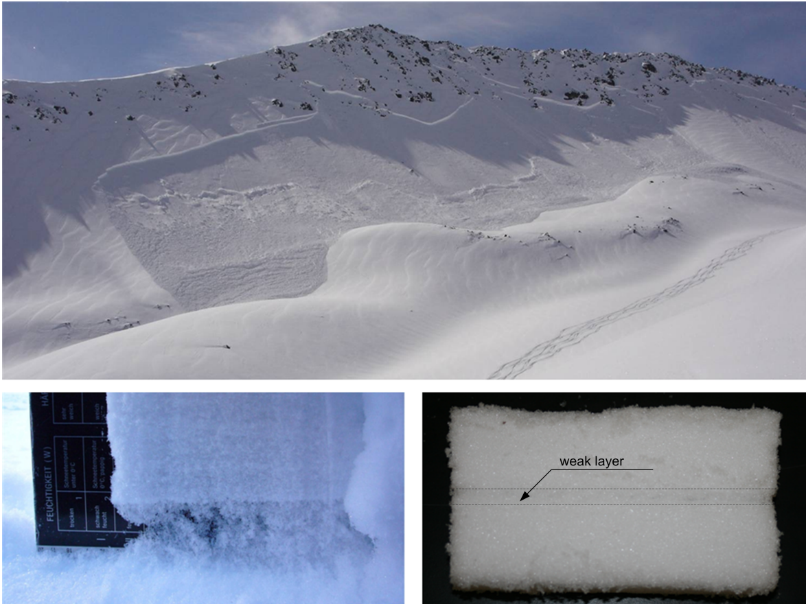
Figure 4.3: From the mountains into the cold lab: (top) dry-snow slab avalanche (Totalphorn, photo: R. Pajarola), (bottom left) natural weak layer (photo: I. Reiweger), (bottom right) artificial weak layer produced in the cold laboratory.
