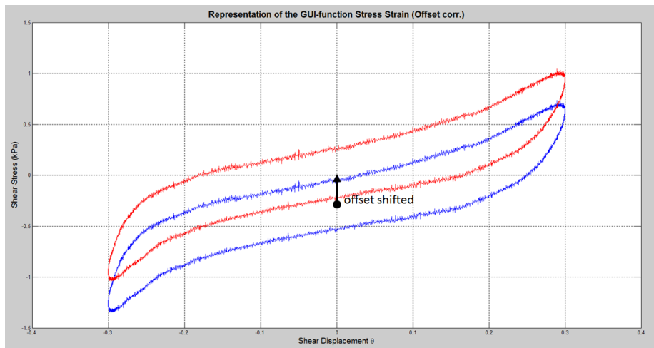
Figure 2.26: Plot of the original dataset of a typical stress-strain curve of a human myocardium in FN -mode at 30% shear displacement (blue) and again with shifted offset (red)
