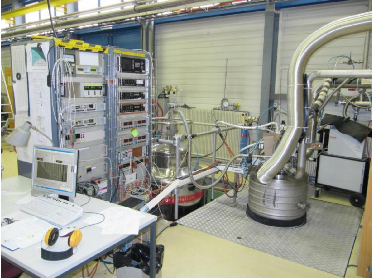
Figure 4.11: The CCDR in operation. The cryostat is placed in the floor, so only the upper part is visible (on the right side of the image). From the dilution refrigerator only the top flange is visible, with all necessary connections (tubes, cables). The tubes of the pump lines are visible, leaving the dilution refrigerator on top and then bending to the right. On the left the electronic module racks are visible as well as the workstation for data acquisition and controlling. The helium dewar for the liquid helium supply for the bath is posed next to the electronic racks, also placed in the ground.
