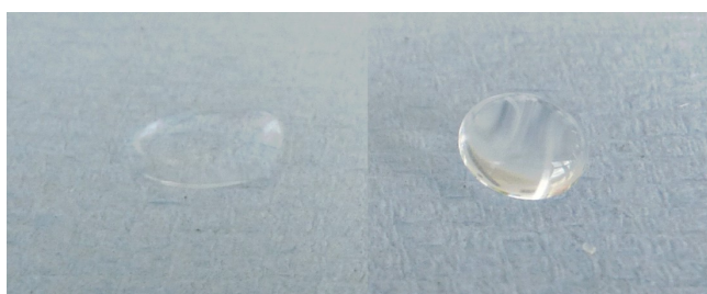
Figure 30: Drop of water on the two surfaces of the protective layer used as the middle layer
