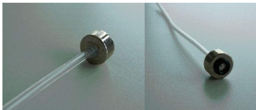
Figure 60: Top (left) and bottom view (right) of the magnetic connector
