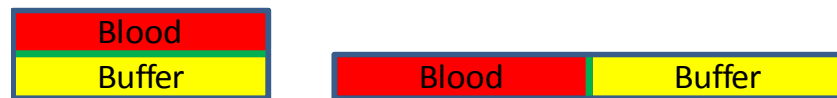
Figure 53: Cross section of the two possible channel configurations; channels on top of each other (left), channels side by side (right), the green line indicates the area available for diffusion
