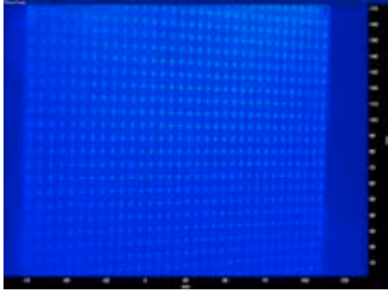
Figure 61: The calibration plate recorded with a Nikon 1.8d lens with aperture 1.8 in a 45° position and 1000mm camera-to-subject distance.
