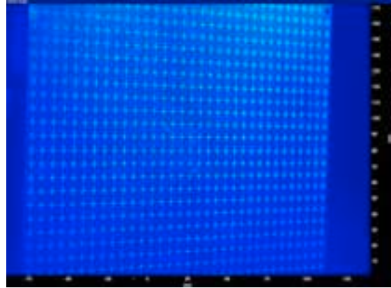
Figure 62: The calibration plate recorded with a Nikon 1.8d lens with aperture 2.8 in a 45° position and 1000mm camera-to-subject distance.
