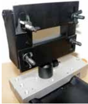
Figure 43: The sheet cleaning beam trap seen from the backside. By loosening the four wing nuts the gap for the laser beam was reduced. The gates were bent towards the laser beam to avoid any double reflection.
