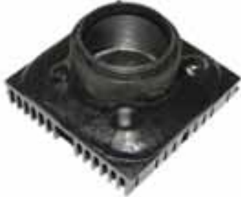
Figure 42: The warm-up beam trap with cooling fins. When both lasers run on full power, the temperature of the device was only slightly above room temperature.
