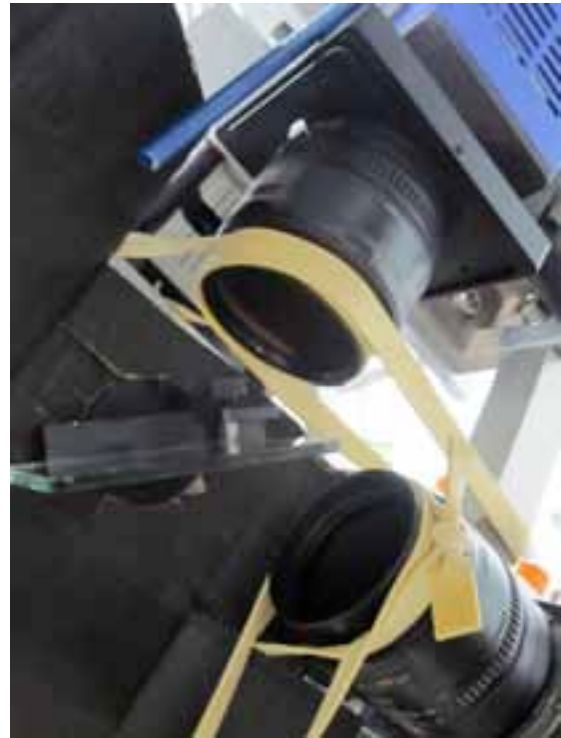
Figure 25: The opened anti-reflection box showing the beam splitter on a rotational mount and the two camera lenses. Camera one (top) had the Scheimpflug adaptor mounted. The rubber bands were necessary for provisional stabilization of the lenses.
