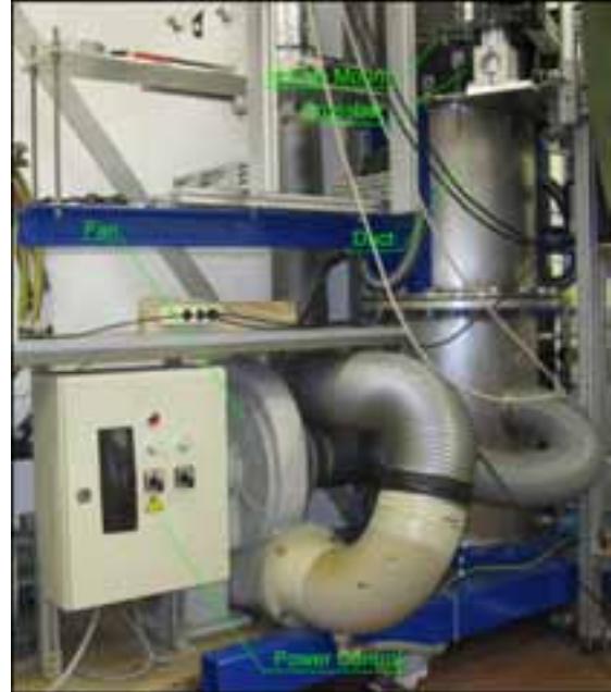
Figure 11: Atmospheric test rig with power control, fan, duct, nozzle mount and crossbar.
