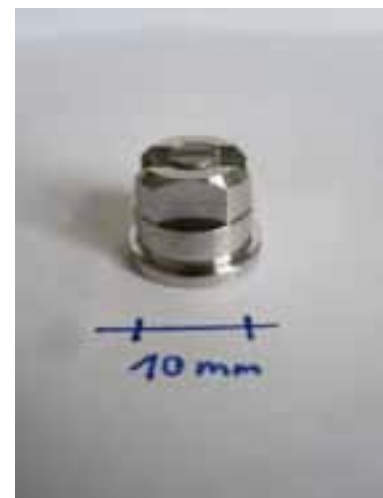
Figure 10: The Le2 nozzle is designed similar to the Le1 only with increase massflow.
