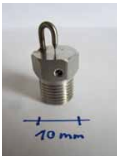
Figure 8: The Mee nozzle with its impaction pin. On the surface of the nozzle, facing the impaction pin, is the orifice measuring 0.15mm in diameter.
