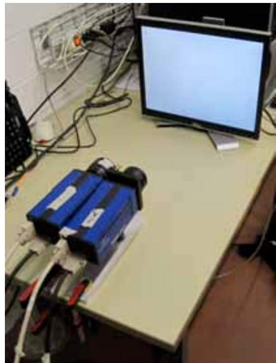
Figure 35: The generation of the white sheet with a computer screen. The LIF camera had the Scheimpflug adaptor mounted.
