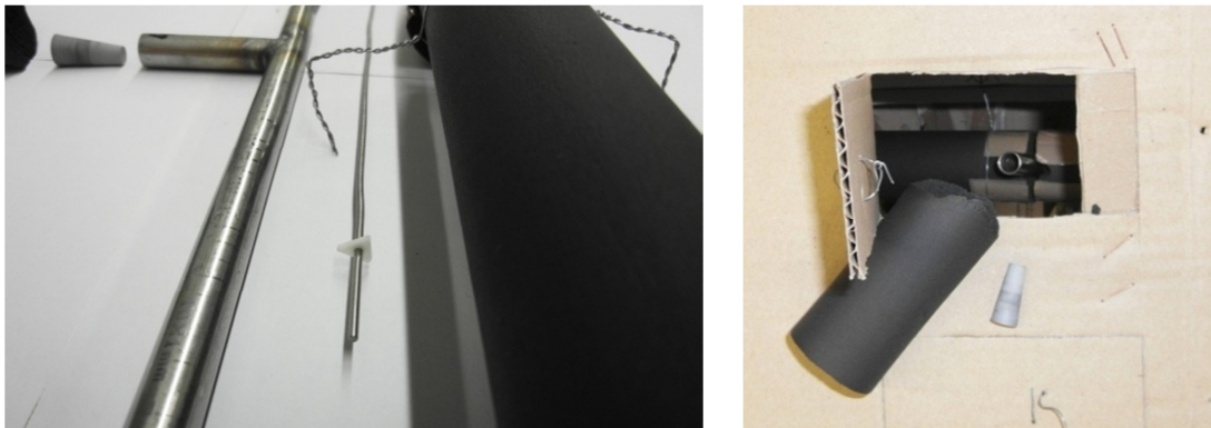
Figure 3-5: Left side picture: close-up of the temperature sensor. positioning in the tube with a spacer made of PTFE located at the upper end of the measuring zone of the sensor to ensure a centric position of the sensor in the tube. Right side picture: access opening in the outer cardboard case for triggering crystallisation (for an overview see figure 3-8) and position of the test tube below.
