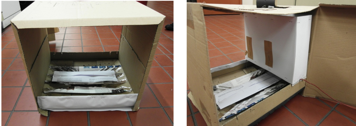
Figure 3-7: Picture on the left side: outer cardboard case (seen from the back side) that exactly fits in the drying oven with cardboard guide slots to enable homogenous distribution of the heated air flow in the oven. In the picture on the right side the position of the inner cardboard case is visible.
