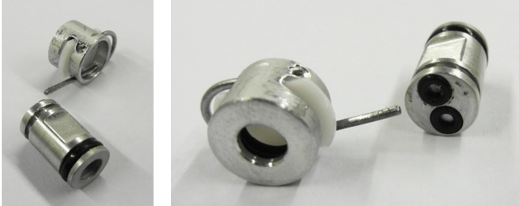
Figure 3-3: Two different views of the triggering valve. In the right side picture the valve body with two axial O-rings is visible. One O-Ring has a small drill to connect the PTFE plate to the tube-inside and the other O-ring contains SA when completely assembled. The other part in the picture is the valve cap with the PTFE plate.
