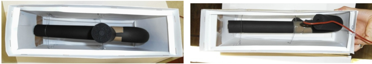
Figure 3-6: Position of the sample tube in the inner cardboard case (fixed with wires) from above (left picture) and from the bottom (right picture).
