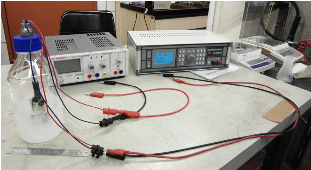
Figure 3-2: Laboratory setup for crystallisation experiments with Peltier-element in the bottle. The pictured Pelteier-unit inside the glass vessel is the first prototype but experimental setup for the final device remained the same.
