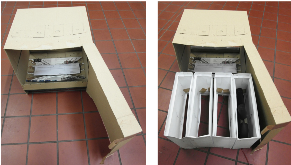
Figure 3-8: Outer cardboard case (seen from the front side) with openings for triggering crystallisation visible on the top (left side picture). The right side picture shows the four inner cardboard cases with a sample tube assembled exemplarily in the rightmost one.
