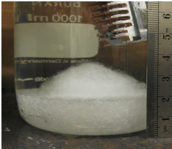
Figure 3-24: The left photo shows the same sample of a SA mixture with 42 wt% water as in the right. It was taken before the pile in the middle dissolved. The rest of the precipitate in the right did not dissolve without slewing.
