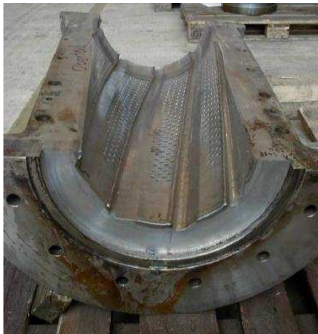
Figure 5: Worn compression housing before refurbishment [ANDRITZ]
