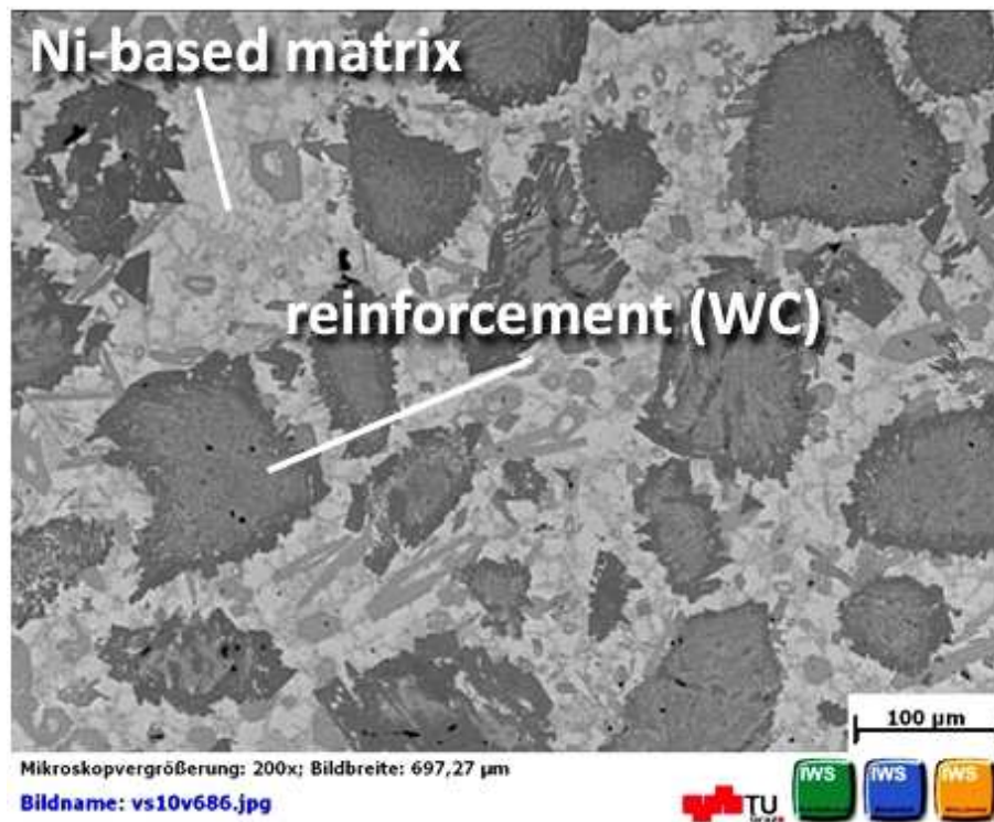
Figure 25: Ni-based matrix with embedded tungsten carbides - specimen_29 (Keraloy)
