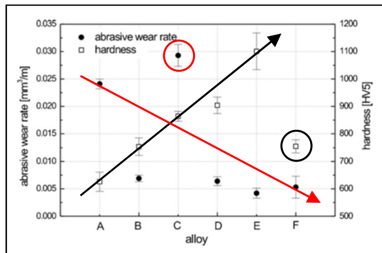
Figure 31: Abrasive wear behavior and hardness for different Alloys A – F in dry sand rubber wheel test [71]
