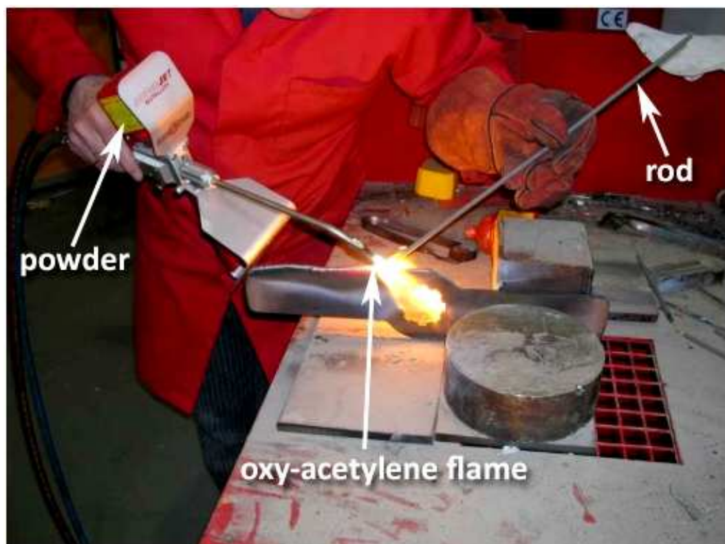
Figure 48: Coating process with Castolin SuperJet-S Eutalloy [89]
