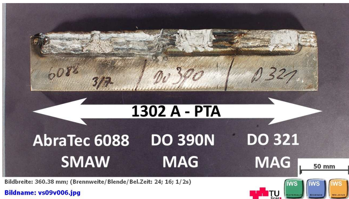
Figure 115: Sample VI – 'hammer fall test'
