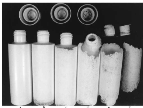
Figure 2-17 Degradation of P(3HB-co-3HV) in aerobic sewage sludge after a: 0; b: 2; c: 4; d: 6; e: 8 weeks. Source: (87).
