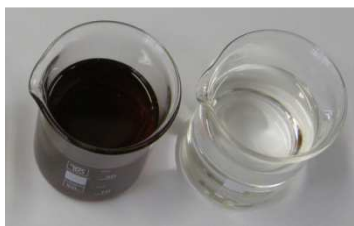
Figure 5-6 CGP from Argent (on the left) and p.a. glycerol (on the right).
