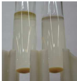
Figure 6-9 Sample tubes after centrifugation. Left: Biodiesel layer visible on top. Right: No Biodiesel layer visible.
