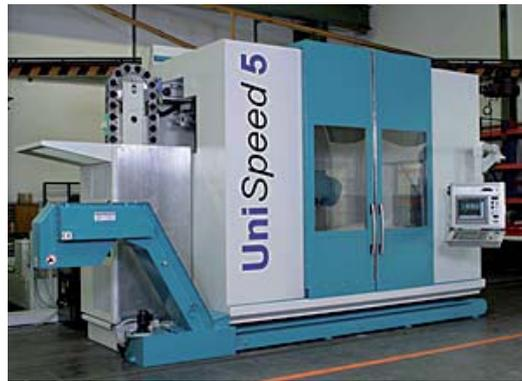
5-Achs CNC Fräsmaschine, [15]
