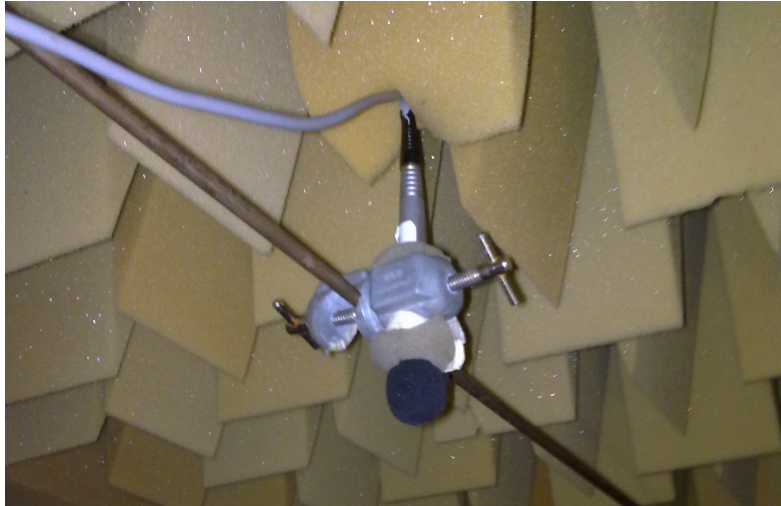
Figure 4.18: Microphone mounted inside the anechoic chamber
