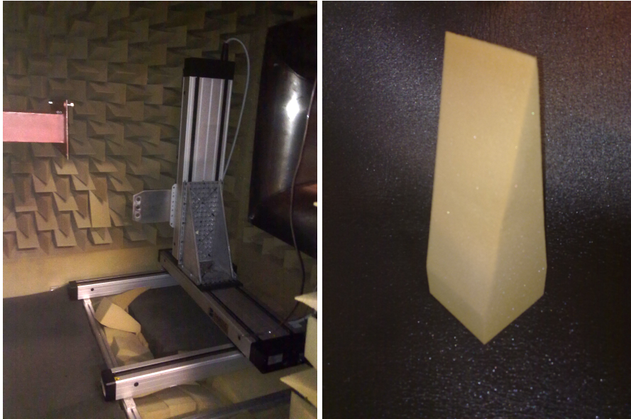
Figure 4.4: Traverse system (left) and sound insulation element (right) of the AWT.
