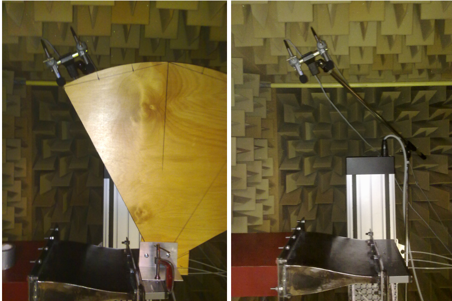
Figure 5.6: Microphones positioned for the directivity measurements, with (left) and without (right) template.
