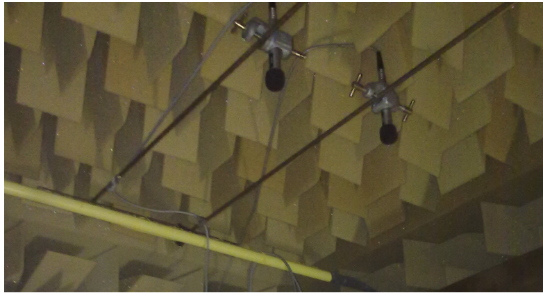
Figure 5.8: Two microphones as they were mounted in the far field tests.
