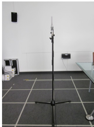
Figure 45: Picture of the used microphone, Behringer ECM8000
