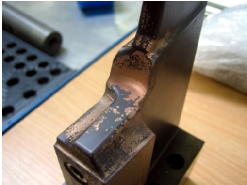
(c) Wear appearance on disassembled TiO protective coated AMPCOLOY® core insert.
