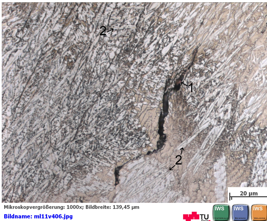
(b) VR0.3.3: Weld metal microstructure and crack detail
