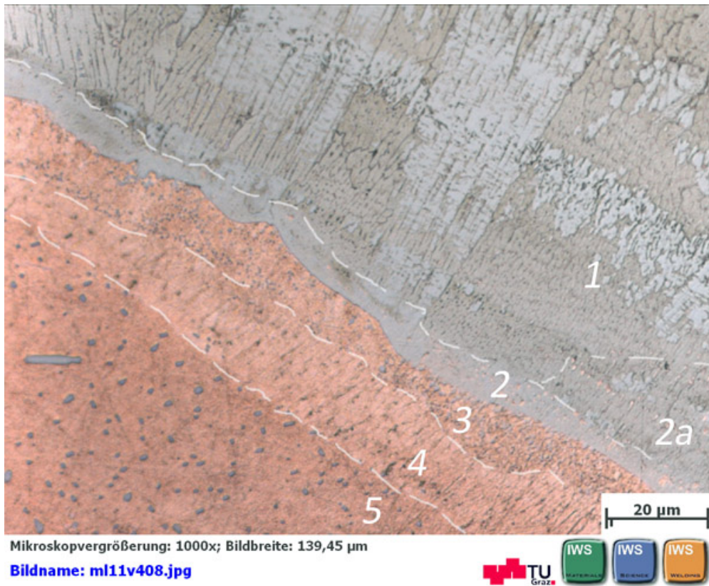
(a) VR0.3.3: optical microscopy of microstructure at the interface.
