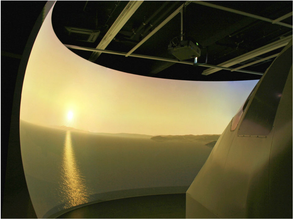
Figure 1.1: Flight simulator I at the TU Graz. Three projectors display the virtual world on a spherical wall with an approximate horizontal field of view of 150^\circ and a vertical field of view of about 33^\circ . The projection wall is approximately 5 meters in front of the pilot. Photo courtesy of Dipl. Ing. Boris-André Prehofer. All rights reserved.
