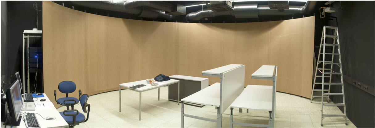
Figure 1.2: The unfinished Flight simulator II at the TU Graz. The cylindrical projection wall has an approximate horizontal field of view of 180^\circ and a vertical field of view of around 44^\circ . The projection wall will be approximately 3.5 meters in front of the pilot.
