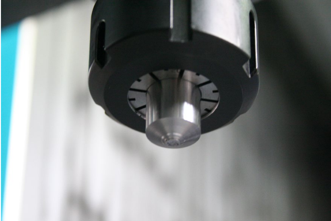
Figure 7.1: Test pin dummy clamped by collet and nut during pilot test sequence
