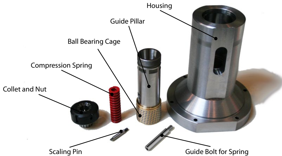
Figure 7.3: Overview of basic components of the tribo-module
