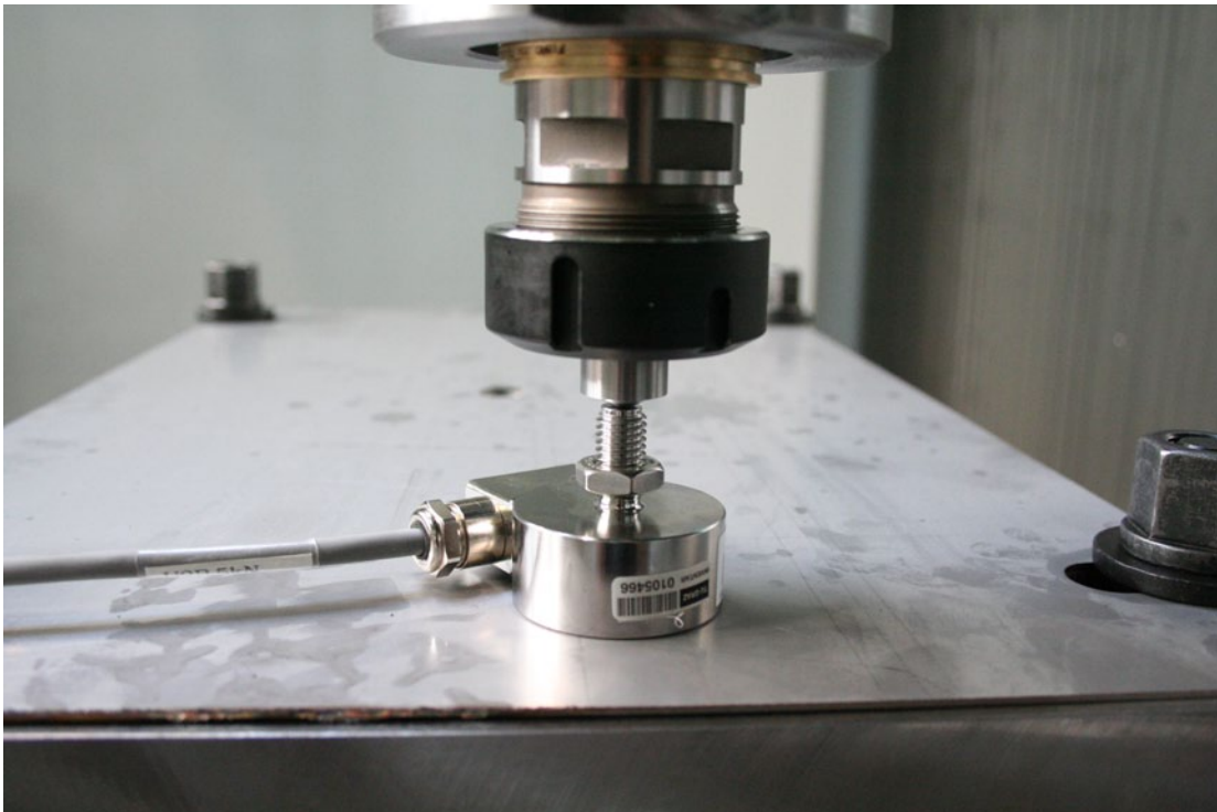
Figure 7.5: Calibration of tribo-module with a load cell
