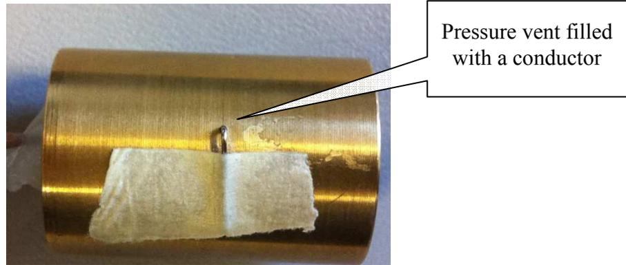
Fig. 3.8 Acoustic coupler with pressure vent
