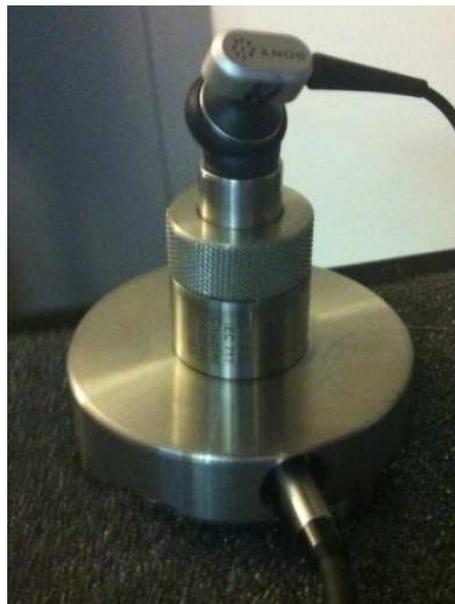
Fig. 3.19 Stand alone IEC 711 standard coupler with IEM
