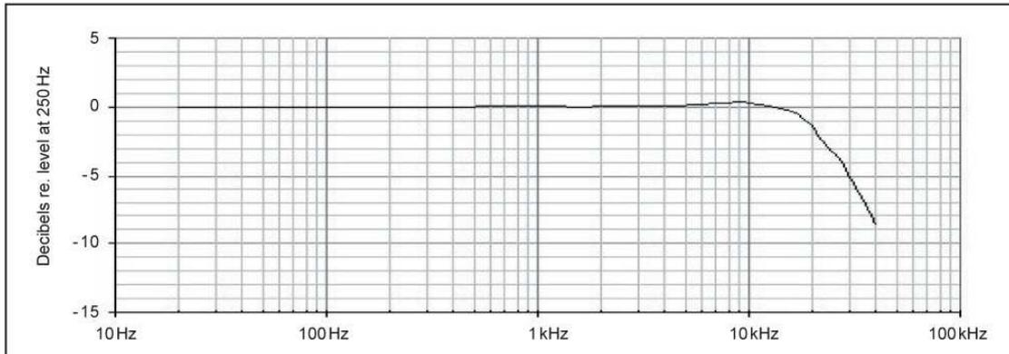
Fig. 2 Typical frequency response for Type 40AG
