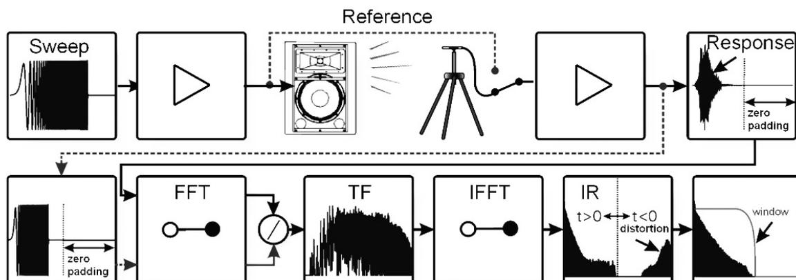
Fig. 4.1 FFT-based impulse response measurements, (Weinzierl, et al., 2009)
