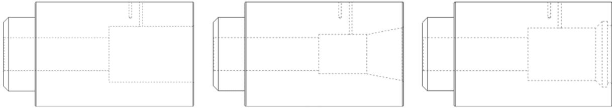
Fig. 5.3 Acoustic Couplers: Type1 (L), Type 2 (M), Type 3 (R)
