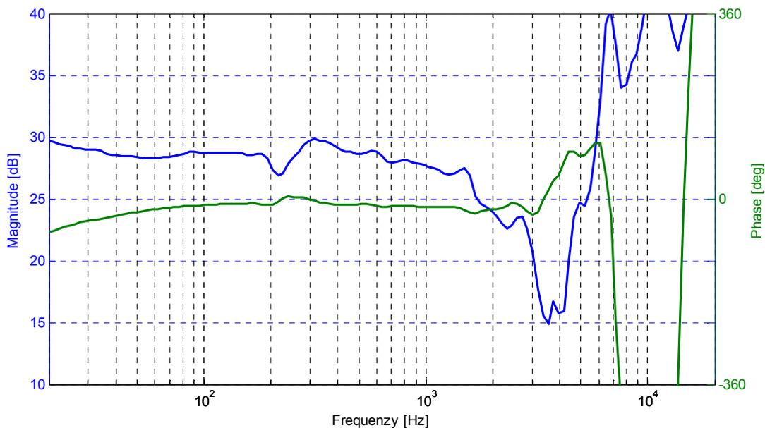
Fig. 2.12 Typical frequency and phase response for a calculated ANC filter
