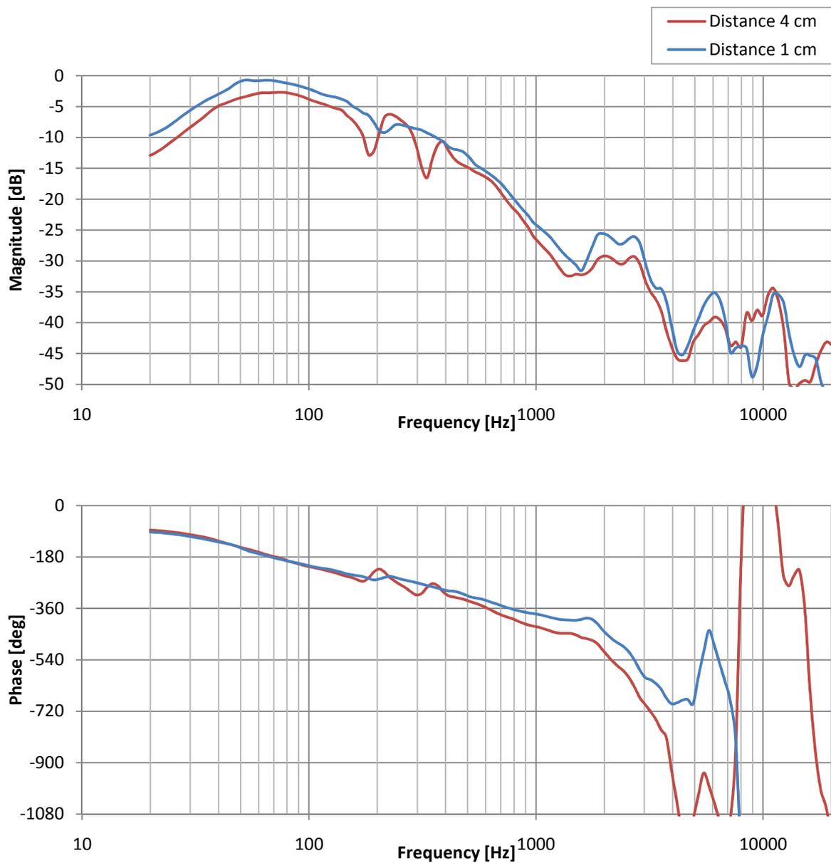
Fig. 3.39 Passive attenuation
