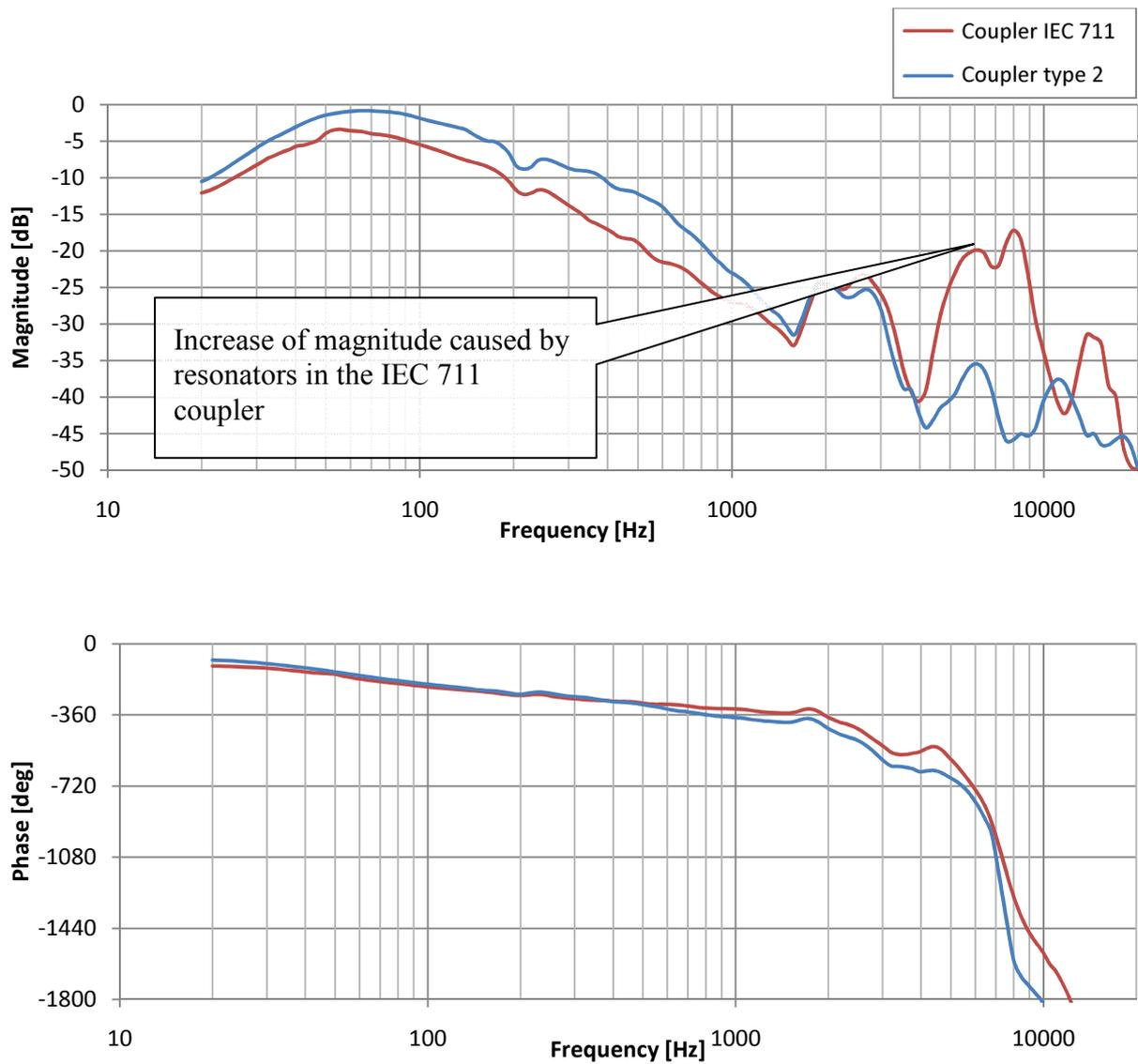
Fig. 3.20 Passive attenuation measurement
