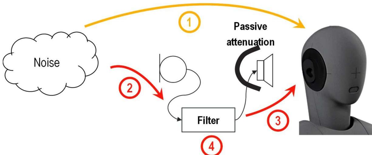
Fig. 2.8 Active and passive noise path
