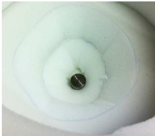
Fig. 3.33 Shape of the absorber material closely to the speaker
