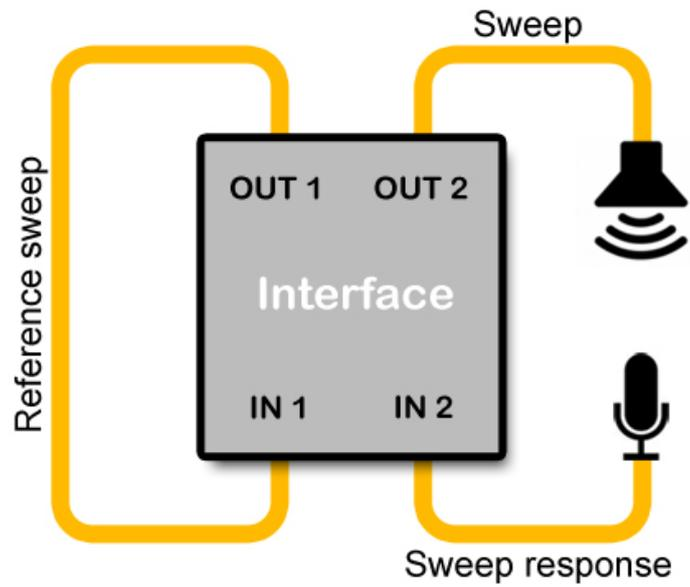
Fig. 4.2 I/O delay compensation
