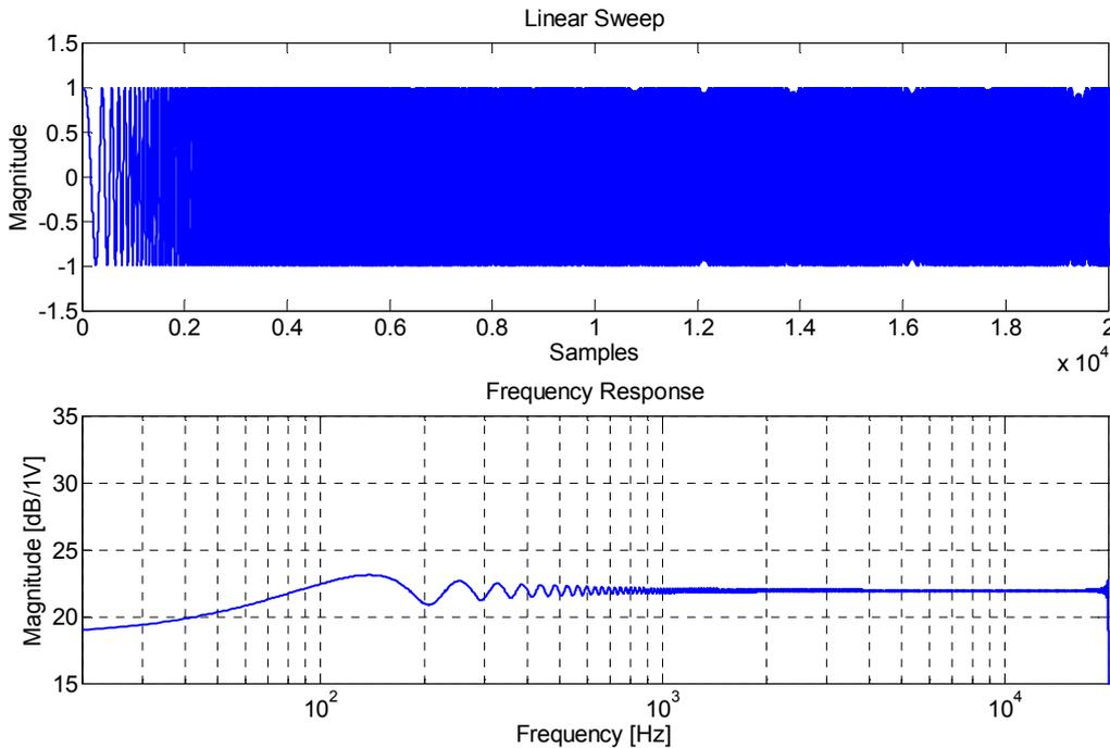
Fig. 2.16 Linear sweep - Time domain (top), Magnitude spectrum (bottom)
