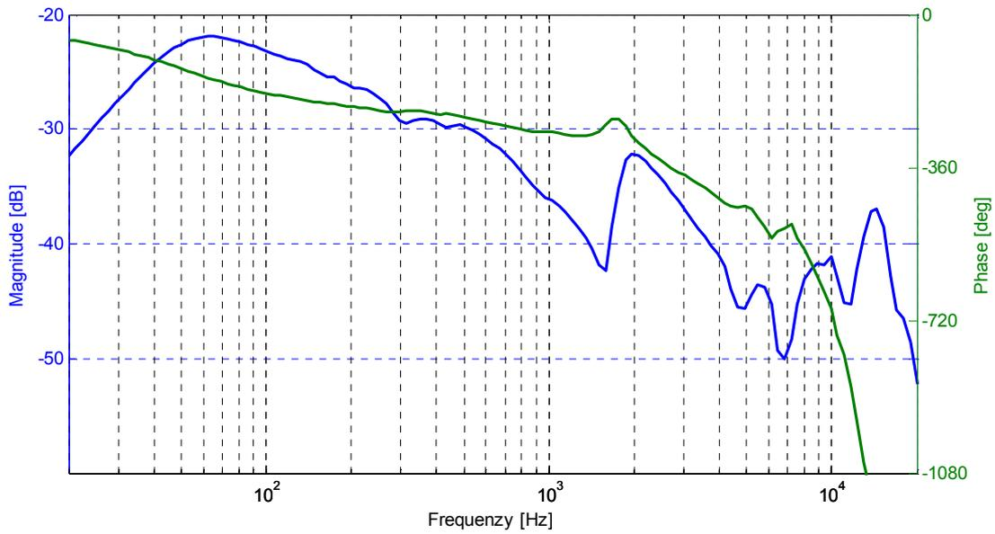
Fig. 2.10 Typical filter gain and phase response, Noise 2 ANC microphone
