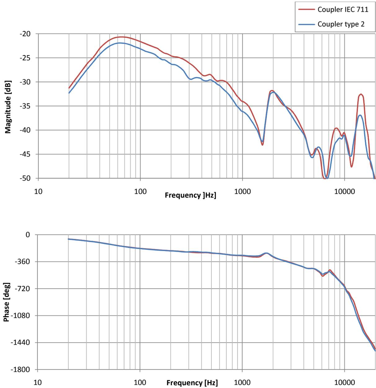
Fig. 3.21 Noise to ANC microphone measurement
