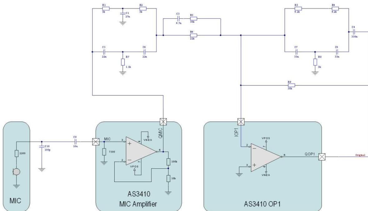
Fig. 2.15 Sample of a filter schematics
