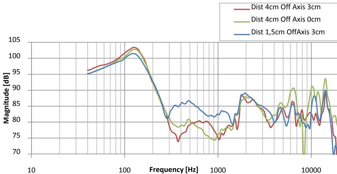
Fig. 3.34 Frequency response in different microphone positions
