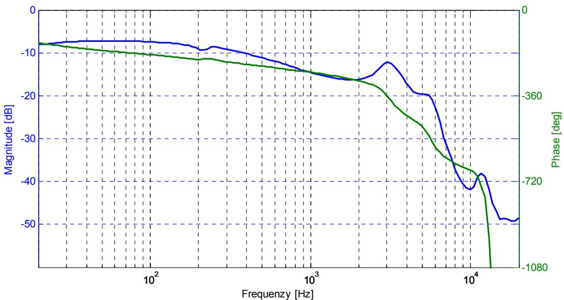
Fig. 2.11 Typical filter gain, Speaker 2 microphone
