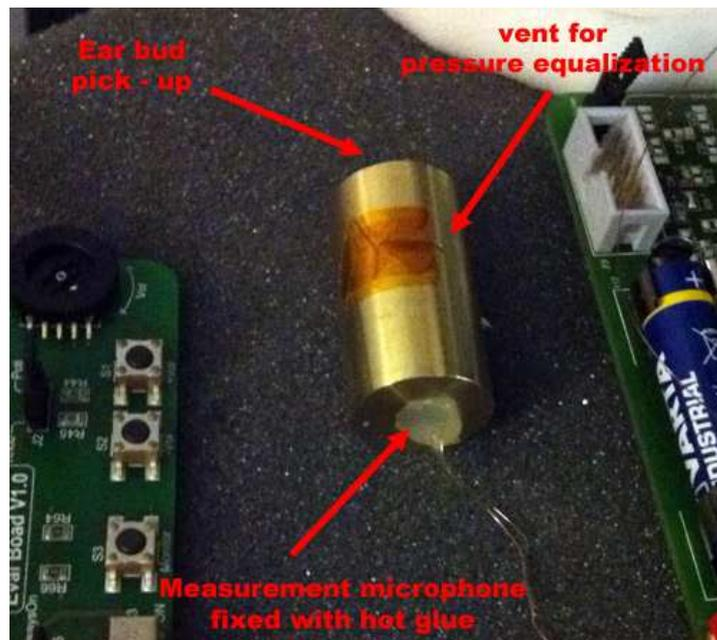
Fig. 3.9 Acoustic coupler, prototype 1 with sealed backside
