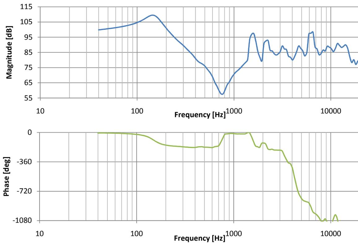
Fig. 3.28 Frequency and phase response of empty measurement box
