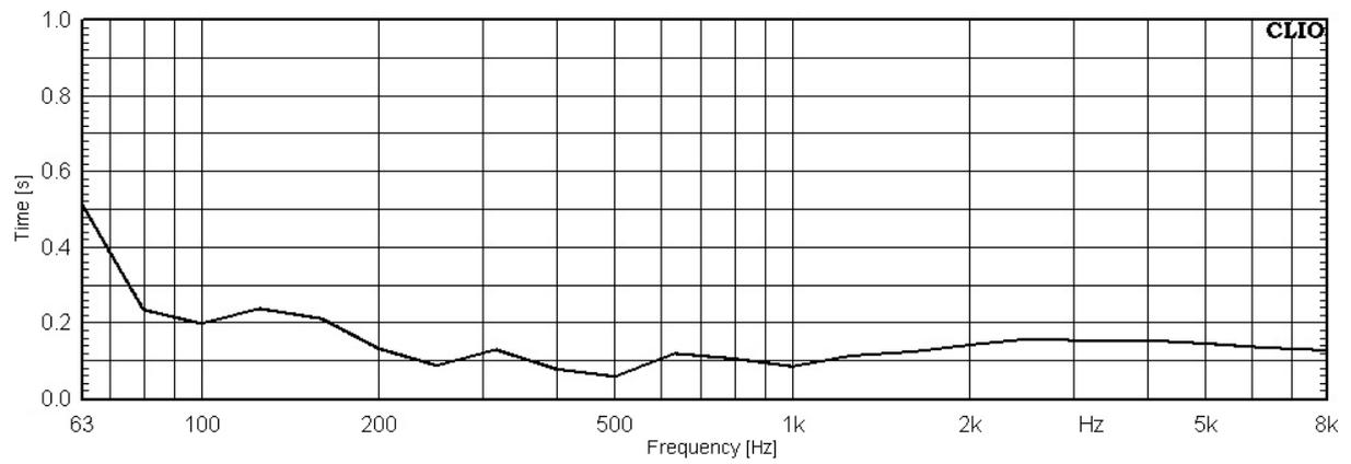
Fig. 3.44 Reverberation time inside the measurement chamber
