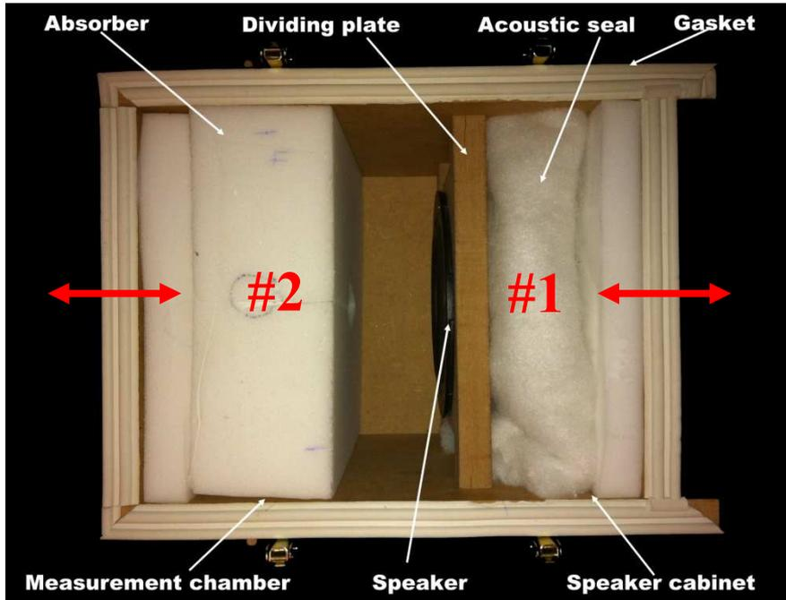
Fig. 3.25 Measurement box inside
