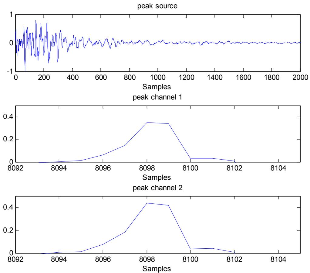
Fig. 4.3 Channel latency between channel 1 and channel 2
