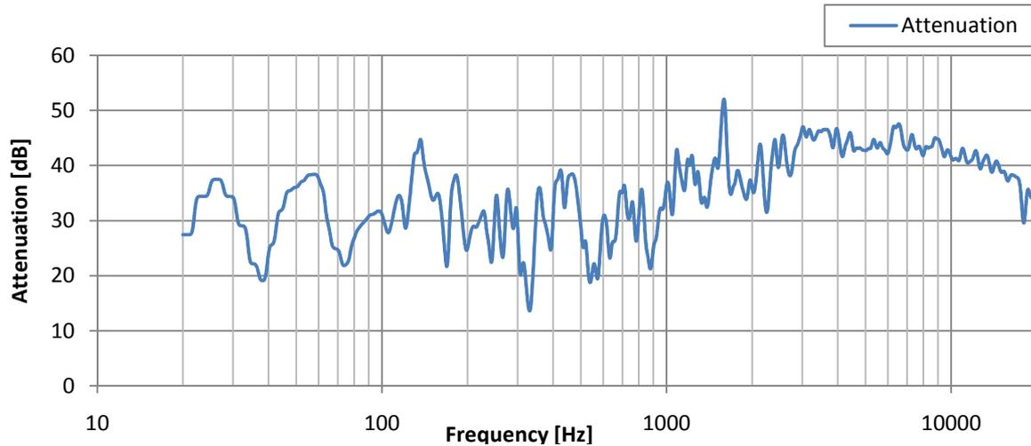
Fig. 3.43 Attenuation from outside to inside the box
