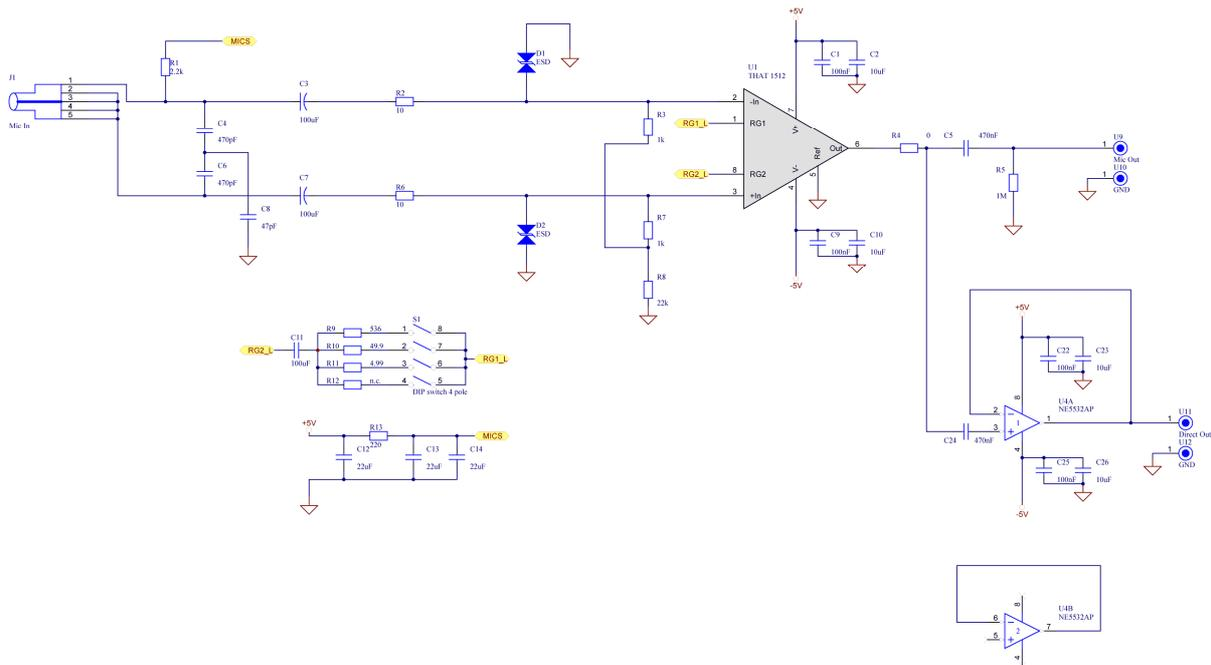
Fig. 3.5 Schematic measurement microphone pre-amplifier
