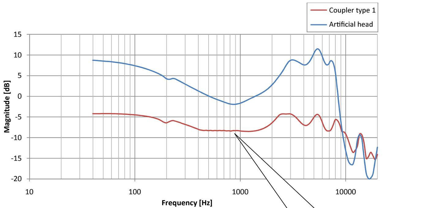
Fig. 3.14 IEM to measurement microphone measurement
