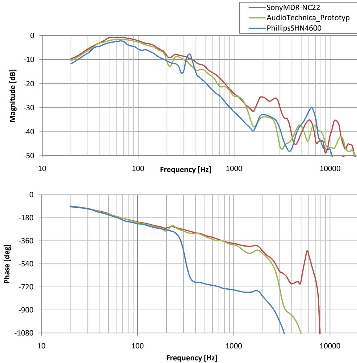
Fig. 3.46 Passive attenuation
