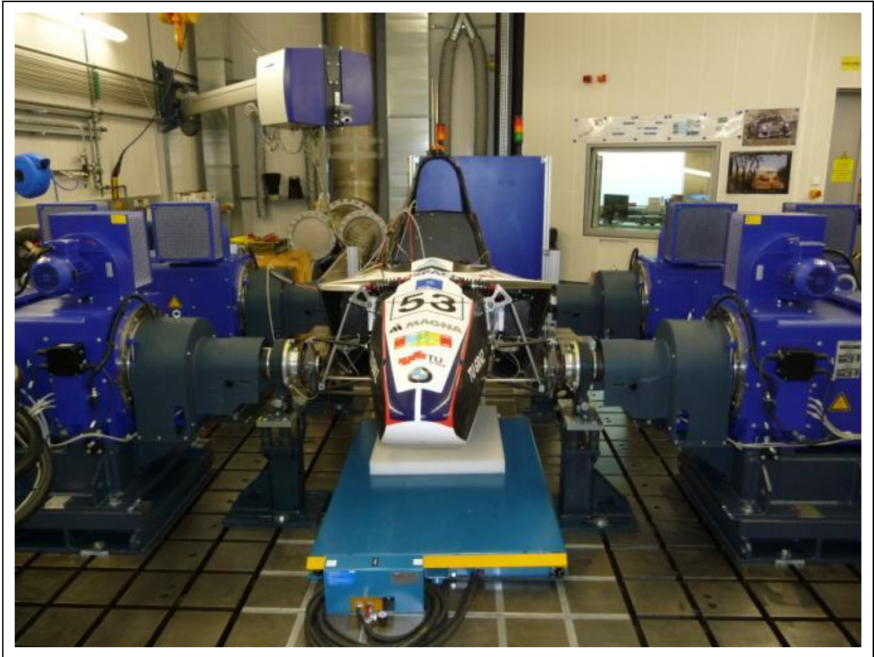
Figure 25: Formula Student vehicle in a HiL configuration 130
