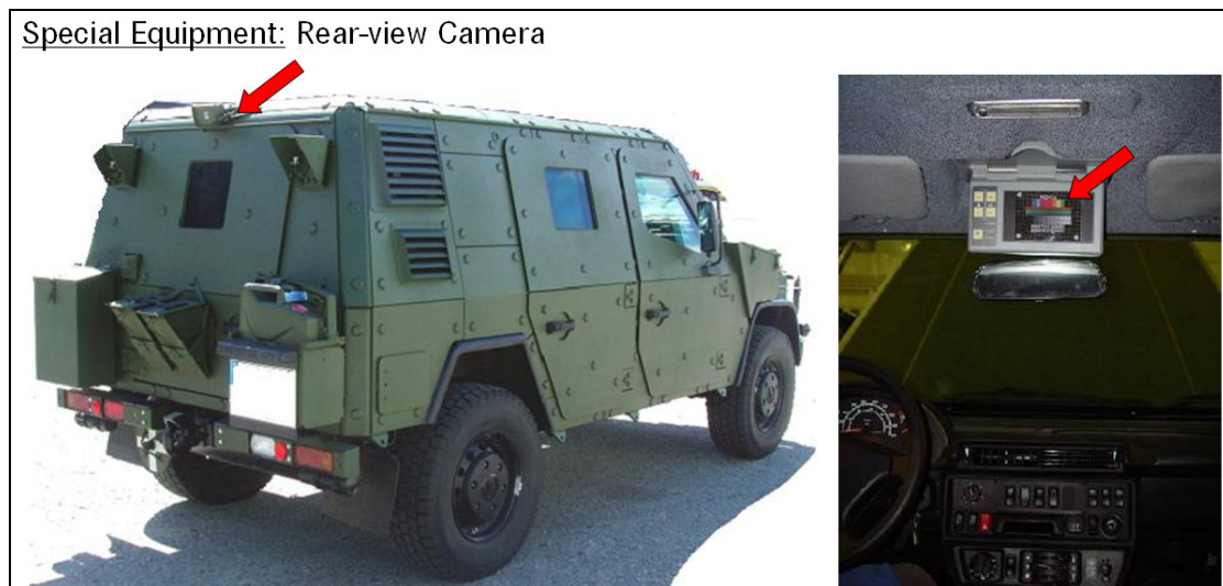
Figure 28: Rear View Camera Installed as Optional Equipment 230
