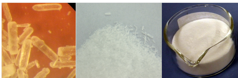
Figure 2.2: Different amounts of acetylic salicylic acid crystals. Isolated crystals, as on the left hand side, are mostly transparent, and show a glossy behavior. In contrast, a legion of crystals, as on the right hand side, has a lot of scattering possibilities, and hence looks uniform and white in all directions.
