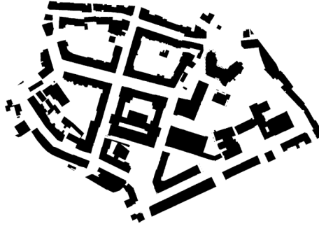
Figure 7.5: Occupancy grid map representing the buildings and obstacles of the environment.
