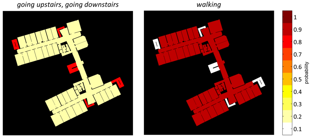
Figure 5.18: Defined probabilities with regard to the current activity. Left: probabilities for going upstairs and going downstairs . Right: probabilities for walking .
