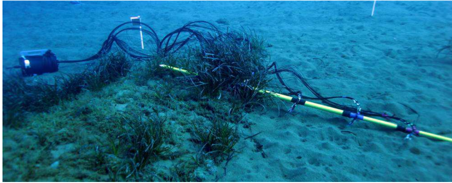
Figure 4.6. MuFO device at the sea ground with fiber bundles positioned over sea grass and sand. (image © HYDRA)
