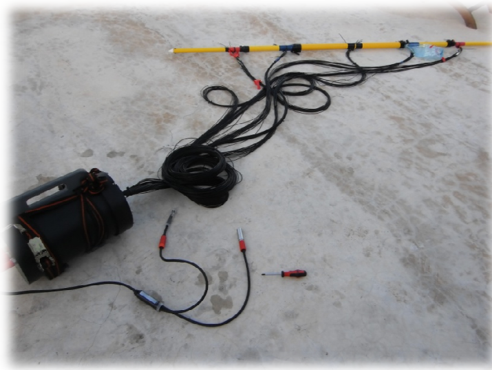
Figure XIII. Optical chemical sensors combined with the multi-branched optical carbon dioxide sensor system (see also chapter 4). 100 optodes positioned on a stick in bundles of 20 fibers each.
