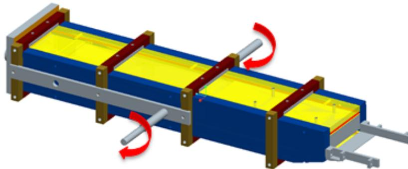
**Figure 4.13** The dewatering unit. The side plates, the bottom and top plate of the channel are made of in transparent polycarbonate. For de-aeration the channel has to be turned from vertical into horizontal position using swivel arms fixed on the frame elements.
