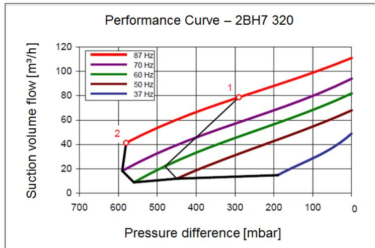
**Figure 4.27** The performance curves of the vacuum fan. At the ordinate axis the suction volume flow in  $m^3/h$  and on the abscissa the pressure difference in  $mbar$  are shown. At a frequency of 87 Hz the achievable suction volume flow is  $110 m^3$  [Rietschle, 2013].
