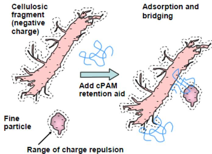
**Figure 2.2** The bridging mechanism onto the surface of a fibre. By adding a high mass cationic polymer with low charge density bridging occurs on the fibre surface. The cationic bridges catch oppositely charged particles [Hubbe et al., 2009].
