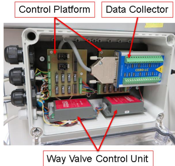
**Figure 4.29** The control platform of the process control system. This platform is the link between the operating elements of the laboratory device and the computer software. The integrated data collector records the pipe pressure of the flow loop and the dewatering zone. The way valve control unit controls the pneumatic pressure switches.
