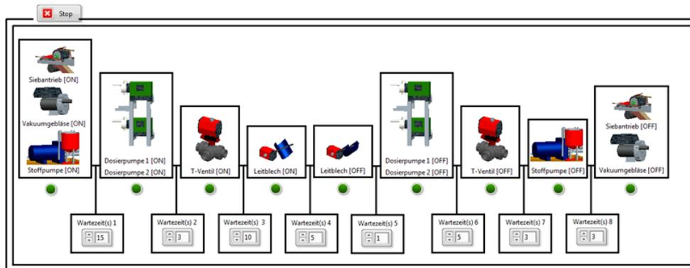
**Figure 5.2** The user interface of the program for an automatic control of the dewatering unit. The control sequence can be divided into nine steps. Between each step the duration of the step can be adjusted in one-second intervals. Sampling of white water takes place between the fourth and fifth step.
