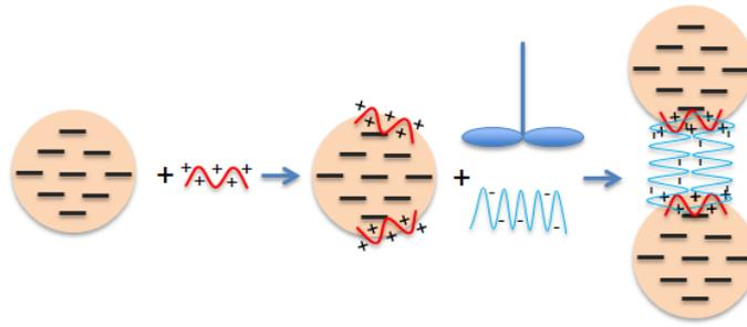
**Figure 2.3** Dual polymer flocculation. The two steps of adding polymers and their influence on flocculation. In the first step a cationic polymer with high charge density is added and patch flocculation occurs. Afterwards the high molecular weight, anionic polymer is added evoking reflocculation by bridging after a shear stage [Svedberg, 2012].
