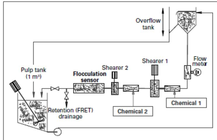
**Figure 3.13** The measuring setup for evaluation of flocculation behaviour. This device is similar to the others introduced, but the suspension flow occurs under static head conditions controlled by a flowmeter. The measurement itself occurs at the flocculation sensor including a transparent rectangular channel, a CCD camera and a light source [Huber et al., 2004].
