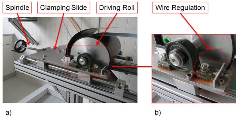
**Figure 4.23** The wire tensioning system. a) The wire tension system includes components as the driving roll, the clamping slide as well as the spindle. To adjust the wire tension the clamping slide is moved using the spindle. b) Using the wire regulation the running direction of the wire is adjusted.
