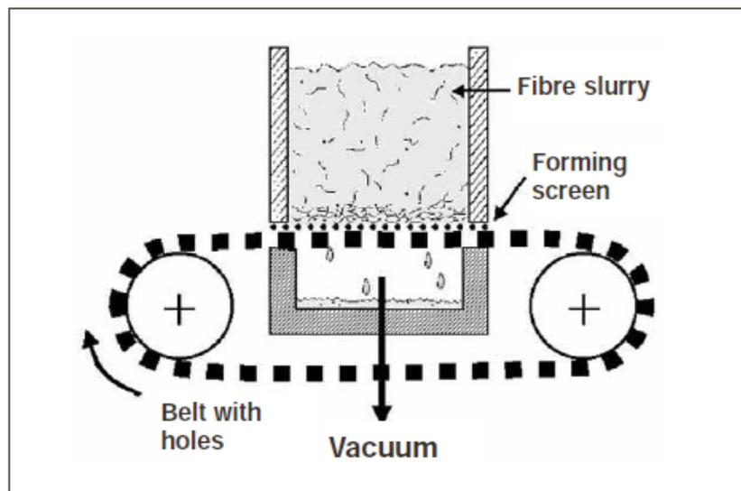
**Figure 3.7** The Moving Belt Former. The mixing chamber is similar to the Britt Jar including an impeller as well as dosage equipment. Beneath a commercial wire a moving perforated and cogged belt as well as a vacuum box support dewatering [Hubbe, 2003].
