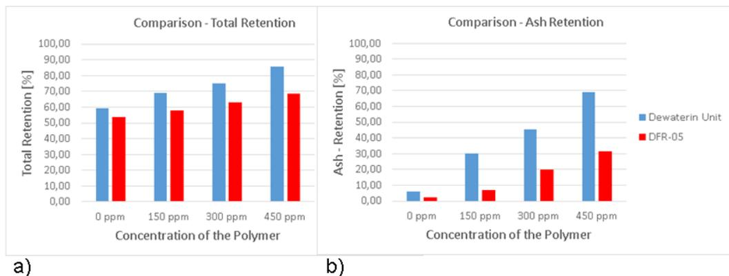
**Figure 5.7** A comparison of retention achieved with the novel device and the commercial tester DFR-05. The results of total retention in a) and of ash retention in b) are quite different. Due to lower turbulences during dewatering the retention achieved with the novel device is clearly higher at each point. Between 0 ppm and 450 ppm the gradient for retention is steeper using the dewatering device.
