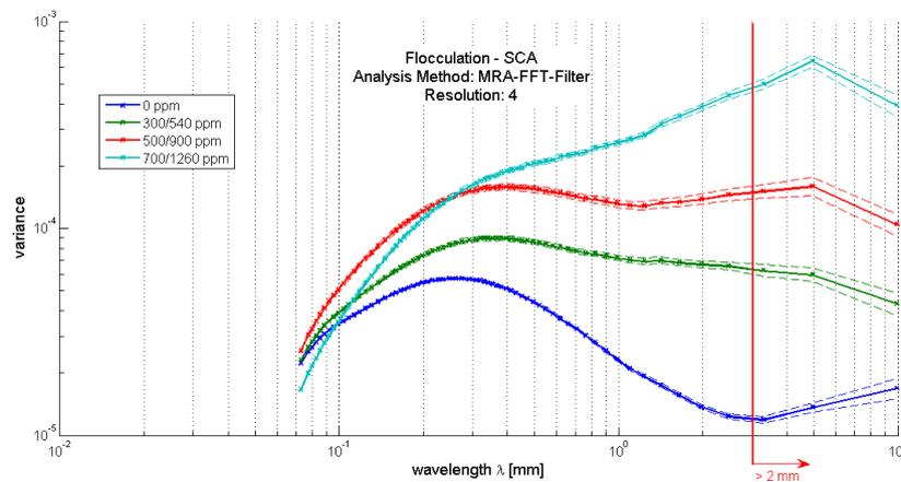
**Figure 6.3** The influence of a dual polymer retention system on the flocculation tendency of a stock sample for SC-A paper. The sample without retention aids (blue graph) clearly shows the lowest flocculation tendency. With the additions of the polymer system, flocculation increases with increasing amount. The strongest flocculation is shown as 700 ppm of PAM followed by 1260 ppm of PVAM are dosed.
