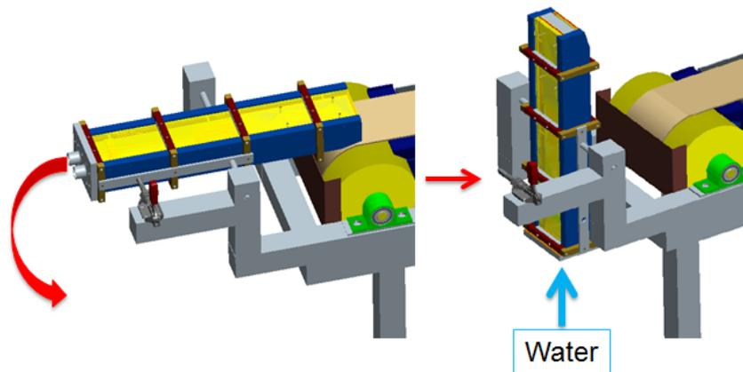
**Figure 4.14** The de-aeration process of the headbox. The headbox is turned from horizontal to a vertical position and is filled up with water.
