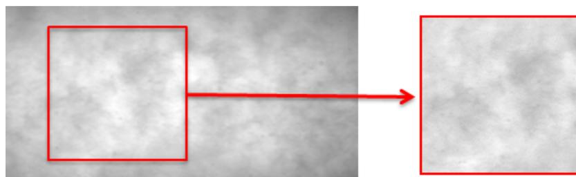
**Figure 4.10** The result after the pretreatment of an acquired image. The pre-treatment, including compensation of uneven illuminations, normalizing of the grey values and cutting into quadratic shape is fully automated.
