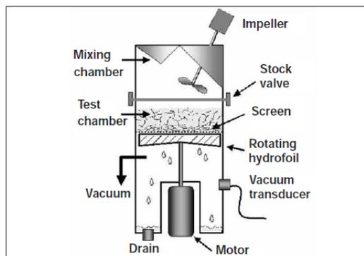
**Figure 3.5** The Pulsed Drainage Device is primarily developed to allow an accurate measurement of newsprint and packaging pulps. The rotating hydrofoil beneath the wire prevents the formation of a fibre mat. By means of two pressure transducers the drainage process can be controlled and data for evaluation of the dewatering behaviour is collected [Sutman, 2000].
