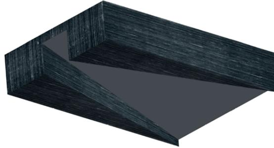
**Figure 4.17** The nozzle with an entire length of 150 mm. The cross section of the nozzle is 35 x 25 mm at the inlet and 100 x 5 mm at the outlet.
