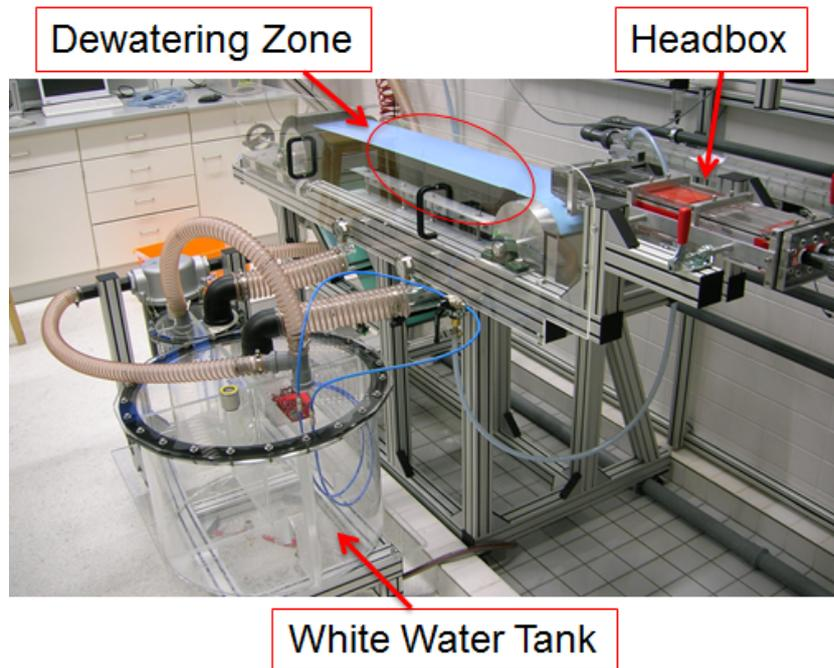
**Figure 4.19** The dewatering device: the fibrous suspension is drained in the vacuum-supported dewatering zone. By means of an air blade the formed fibre web is removed after dewatering. The installed wire cleaning equipment cleans and dries the wire. The produced white water is stored in transparent white water tanks.
