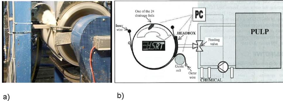
**Figure 3.10** The twin wire retention tester represents a methodology to simulate drainage and retention behaviour prevailing in gap formers. a) The cylindrical frame with the two wires and the rotating headbox are shown. b) A schematic diagram of the device including the dosing points [Sivén and Manner, 2000].
