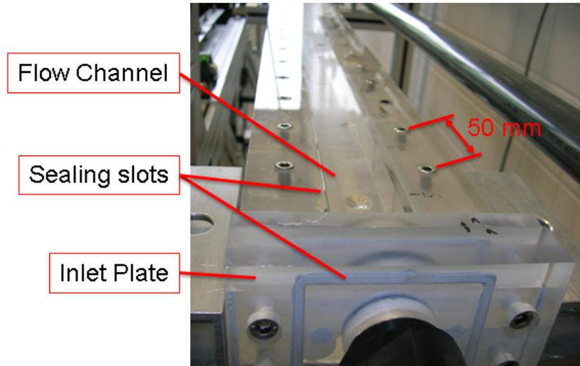
**Figure 4.8** The observation channel in more detail. The material used for the transparent design is polycarbonate. The sealing is achieved by slots in which a sponge rubber is placed and pressed onto the counter-plate.
