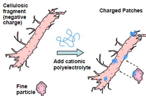
**Figure 2.1** The patch mechanism on the surface of a fibre. By adding a cationic polymer of high charge density and low molecular weight patches are formed on the fibre surface. These cationic patches attract oppositely charged particles [Hubbe et al., 2009].
