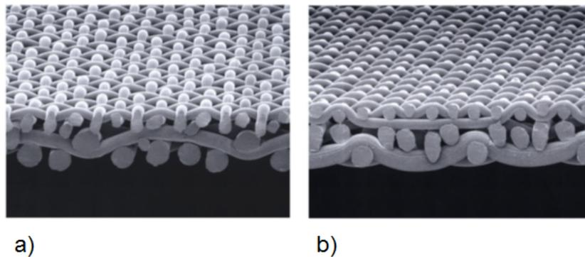
**Figure 4.22** The structure of the *GeoflexX – Change* a commercial drainage wire manufactured by *Andritz – Kufferath*. In a) the warp or longitudinal threads; b) the transversal direction of the drainage wire.
