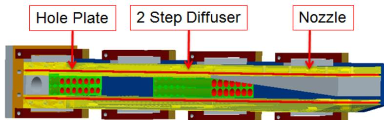
**Figure 4.15** The first version of built-in components. The components are a hole plate used to distribute and accelerate the suspension, a two-step diffuser to accelerate the suspension and to generate turbulences at the end as well as a wedge-shaped nozzle.
