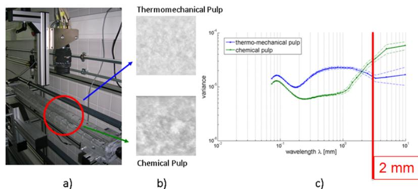
**Figure 4.11** The measurement of the flocculation behaviour. a) The measurement setup is illustrated, in b) the acquired images after pre-treatment of two different samples are shown and in figure c) the results achieved by image analysis are presented. Above a wavelength of 2 mm the detected structures can be considered as flocs, the chemical pulp shows a tendency to build large flocs.
