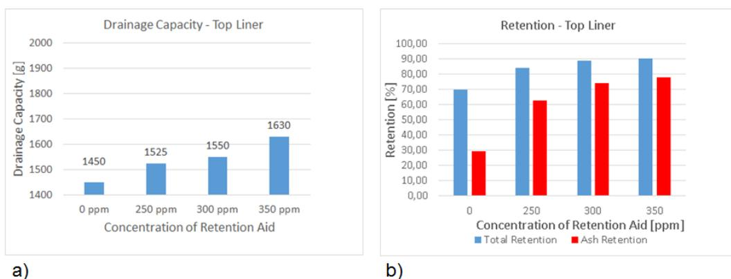
**Figure 6.6** The drainage capacity as well as the retention evaluated for the test liner sample. The higher the concentration of the dosed retention aid the higher are both the total retention and ash retention.
