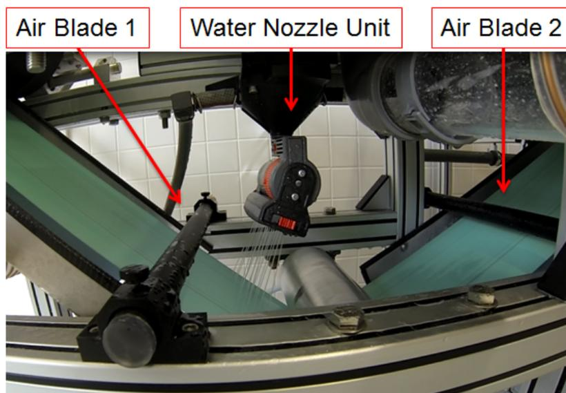
**Figure 4.24** The wire cleaning unit. This equipment consists of two air blades with hole perforation and a water nozzle unit. By means of the cleaning equipment uniform wire conditions at the headbox can be achieved.
