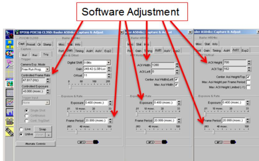
**Figure 4.9** A part of the operator window of the image acquisition software. The shown values for frame rate, gain, exposure time, and scan size are used for the measurements in the flocculation unit.
