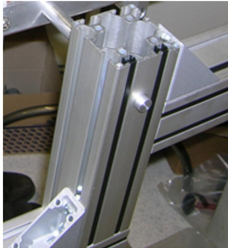
**Figure 4.20** The aluminium profile used for the frame of the dewatering unit is presented. This quadratic shaped profile enables an easy assembly and handling.
