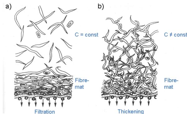
**Figure 2.5** The difference between filtration and thickening. a) The filtration mechanism. There is a sharp division between the formed fibre mat and the suspension. b) The thickening mechanism. In comparison to filtration there is no division, the concentration of the built up fibre mat decreases continuously [Bos et al., 2006].
