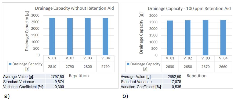
**Figure 5.3** Evaluation of the reproducibility of drainage capacity. a) Drainage capacity without retention aids. The value of the variation coefficient is 0.003 %. b) The results of drainage capacity measured when dosing a retention aid. The variation coefficient is 0.006 %. In summary the measurement of drainage capacity show a high level of reproducibility.
