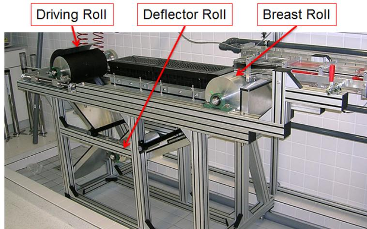
**Figure 4.21** The rolls supporting the drainage wire. The dewatering device includes three rolls; the breast roll, the rubberised and convexly arched driving roll and the small deflector roll positioned beneath the suction boxes.
