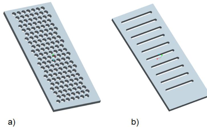
**Figure 4.26** a) The perforated plate used in each drainage box. The shifting of the lines of holes assure an uniform drainage as the open area is equal in every line in length direction. b) An alternative drainage plate designed with slots. The open drainage area is reduced by 50 percent.
