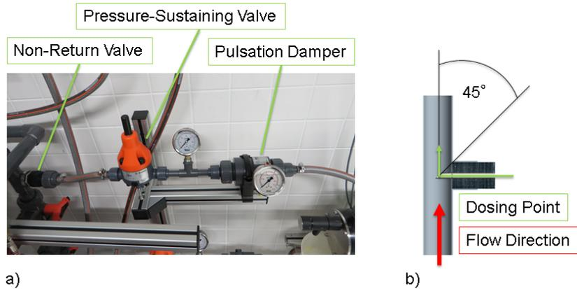
**Figure 4.6** a) The elements of the dosing unit. These elements are the pulsation damper, the pressure sustaining valve and the non-return valve. These three elements are necessary to prevent volume fluctuations caused by pulsations. b) The points of dosage in the pipe are shown in more detail. The injection needle of the non-return valve is positioned in the centre of the pipe to achieve a homogeneous distribution of the dosed additives.
