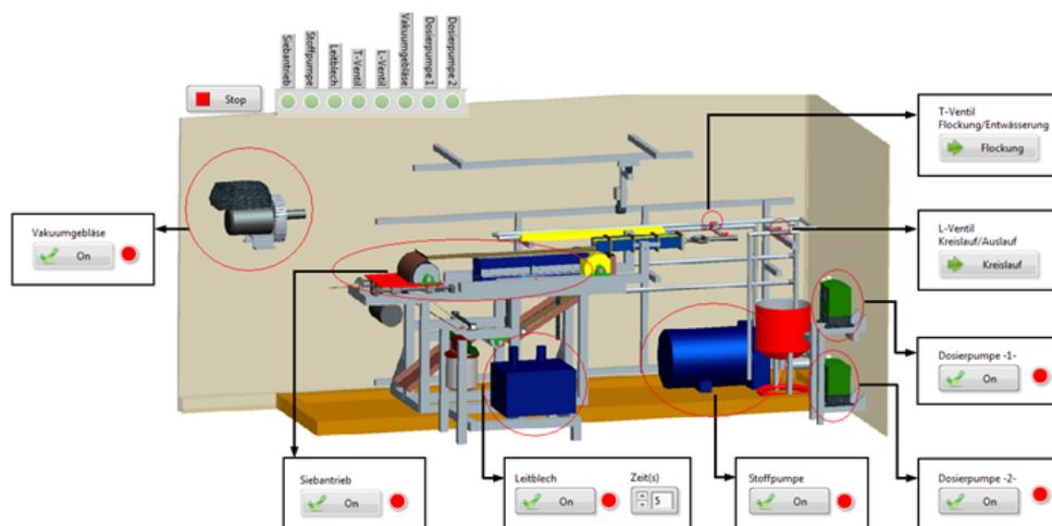
**Figure 4.30** The user interface of the process control system. The design drawing illustrates the whole laboratory device and gives an overview of the controllable elements. Each element is linked with an on- and off switch as well as an coloured button which signals the operating state. The sampling unit in the white water tank is additionally equipped with a timing unit.
