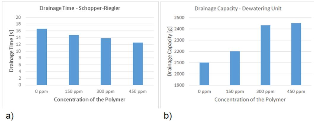
**Figure 5.6** a) The drainage time (Schopper-Riegler) of the fibrous suspension. These results clearly show a decreasing drainage time due to an increasing amount of polymer. b) The drainage capacity in g measured via the dewatering unit is presented. Because of an increasing polymer concentration the drainage capacity of the fibrous suspension increases too.
