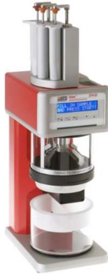
**Figure 3.4** The DFR- Tester developed by BTG Instruments enables an independent measurement of retention, dewatering and freeness. The measurement is performed without support of vacuum and with or without agitation. A scale is used to control the drainage process and to detect filtrate quantity over time. The collected data is plotted in a diagram [BTG-Instruments, 2010].
