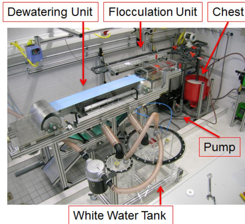
**Figure 4.2** The measurement setup of the novel device. The suspension is stored in the pulp chest with a volume of 40 litres. Using a centrifugal pump the suspension is transported to the flocculation unit and the dewatering unit.
