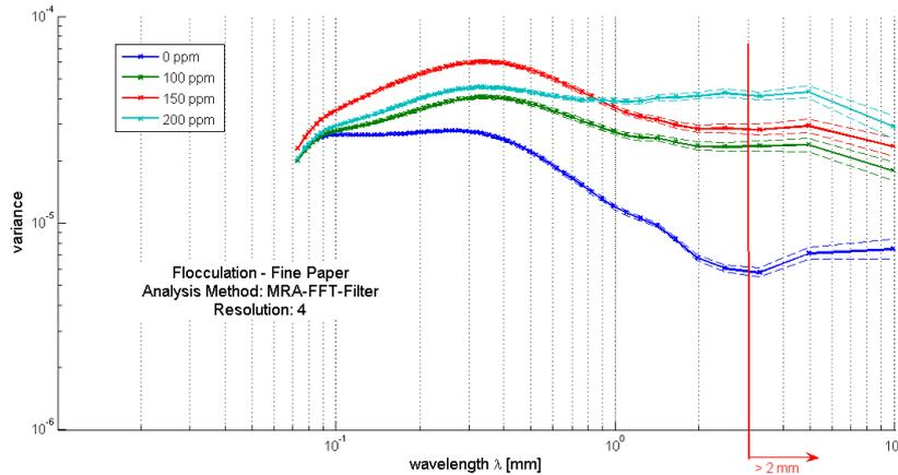
**Figure 6.1** The influence of polymer concentration on the flocculation behaviour of the given suspension. The retention system clearly increases flocculation with increasing effect of increased polyacrylamide dosage.
