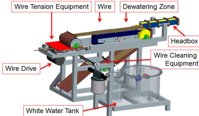
**Figure 4.12** The dewatering unit. This unit consists of a headbox, a drainage wire, a vacuum supported dewatering zone, a wire tension equipment, a wire drive, a cleaning equipment as well as a white water tank.
