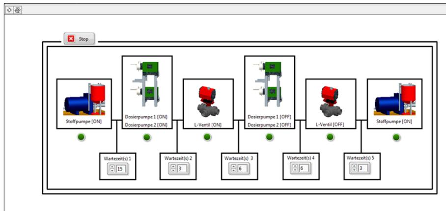
**Figure 5.1** The user interface for an automated measurement of flocculation. The automated sequence is divided into six steps and starts with the activation of the centrifugal pump, the dosing pump, the L- ball valve followed by the deactivation of the dosing pump, the L- ball valve and the centrifugal pump. The time between each step of the sequence can be adjusted in one-second intervals via additional control panels located between the symbols .
