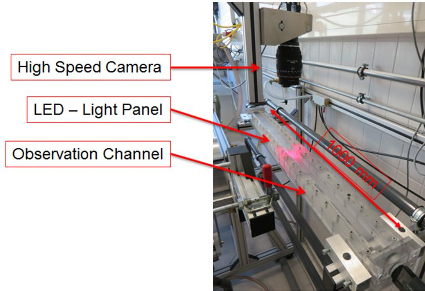
**Figure 4.7** The flocculation unit consisting of an observation channel, a high speed camera and a LED-light panel. Using this equipment images of the flowing suspension are acquired.
