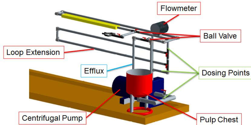
**Figure 4.3** The most important basic elements of the novel laboratory device. Elements necessary for the transport in the loop are marked red, the green marked elements are important for dosing additives. When chemicals are dosed, the suspension leaves the closed loop through the blue marked efflux.
