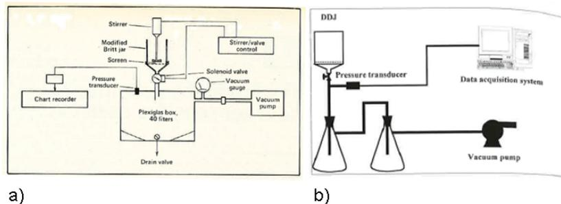
**Figure 3.3** a) The Retention and Drainage Tester. The principle of measurement is similar the DDA. By means of two independent modes of testing drainage without agitation and vacuum support as well as dewatering and retention under the influence of vacuum and agitation are possible [Abson et al., 1980].
