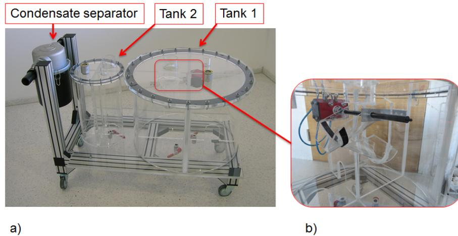
**Figure 4.28** a) The white water tanks of the dewatering device. Each drainage box is connected to one of these tanks. For vacuum-supported dewatering the tanks are supplied with vacuum generated by one vacuum pump. The condensate separator is used to protect the vacuum fan from fluid particles of the white water. b) The equipment for sampling the white water. As soon as constant drainage conditions are achieved the white water is directed in a separate compartment.
