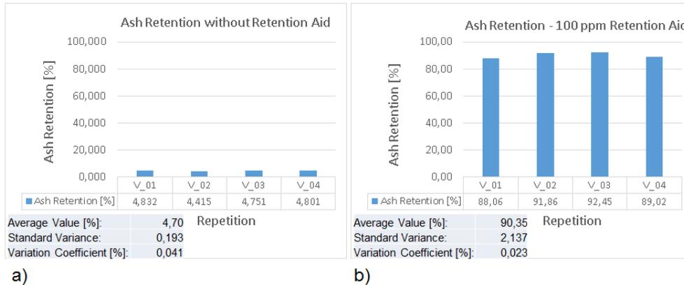
**Figure 5.5** Reproducibility of the measurement of ash-retention. a) The results of ash-retention of the suspension without adding retention aids. An average value of ash-retention of 4.7% and a variation coefficient of 0.04% are reached. b) Ash-retention reached using retention aids. An average value of about 90% and a variation coefficient of 0.02% are reached.
