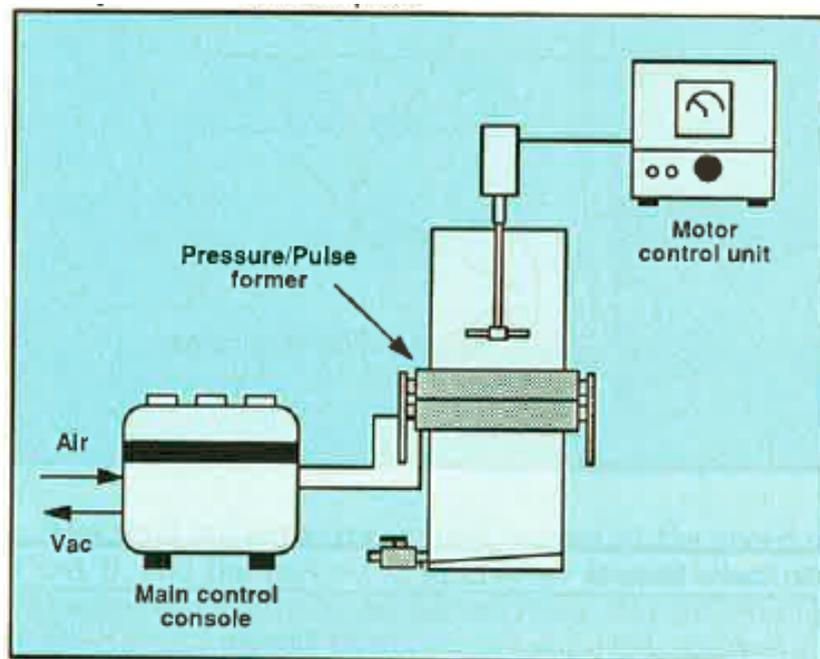
**Figure 3.8** The turbulent pulse sheet former represents a modification of a standard handsheet former [Staib, 1991].
