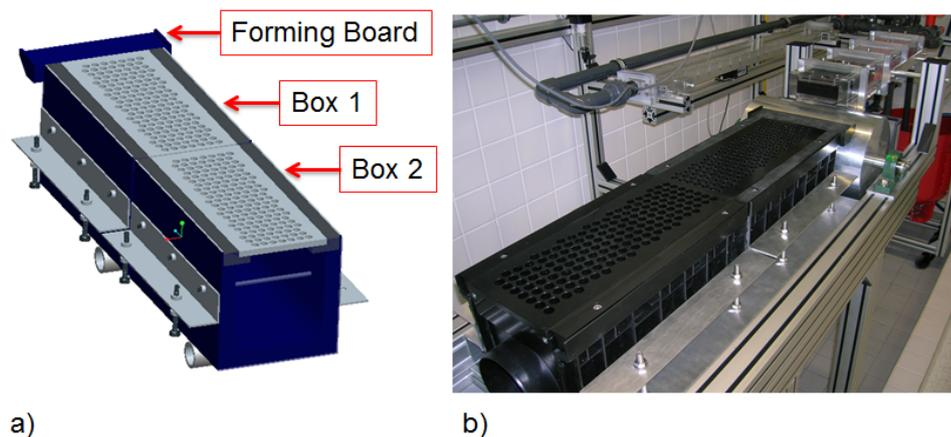
**Figure 4.25** a) Schematic design of the drainage zone. The unit consists of a forming board and two drainage boxes. The boxes are covered by perforated drainage plates. b) The construction of the dewatering unit. Threaded rods are used for height adjustment of the boxes to achieve a uniform contact with the drainage wire.
