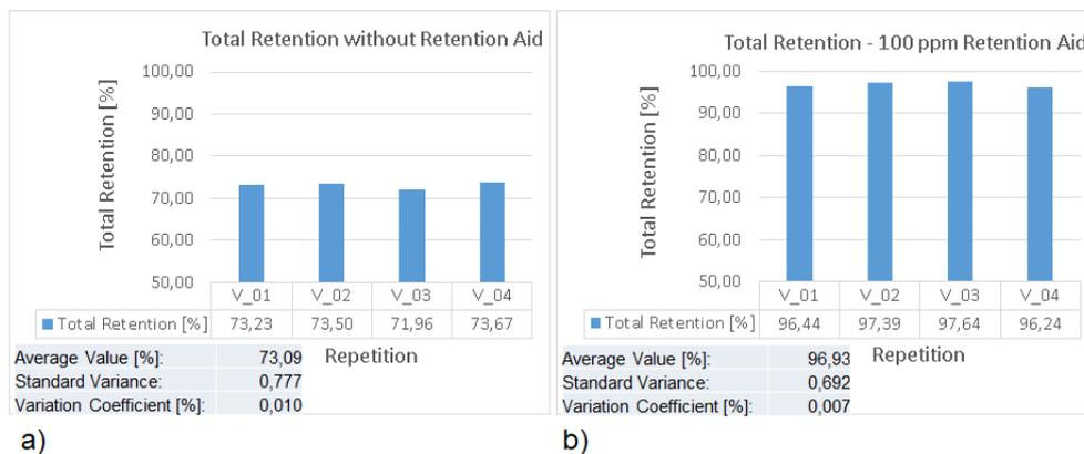
**Figure 5.4** Evaluation of the reproducibility of the measurement of retention. a) Total Retention without additives. The average value of four trials is 73% and the variation coefficient is 0.01%. b) Total Retention when adding retention aids. The average retention value increases to 96%, a variation coefficient of 0.007 is reached.
