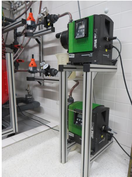
**Figure 4.5** The entire dosage unit. The dosing pumps used for the laboratory device are called DME 150 manufactured by Grundfos. The dosing capacity of the DME 150 is in the range of 20 *ml/h* up to 150 *l/h*.
