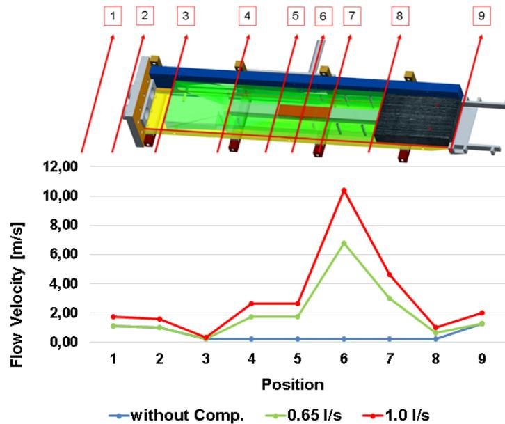
**Figure 4.18** The velocity profile of the designed headbox. The green graph illustrates the velocity profile at a flow rate of 0.65 l/s. The profile reached at a maximum flow rate of 1 l/s is shown by the red graph. For comparison the blue graph illustrates the profile without any built-in components.
