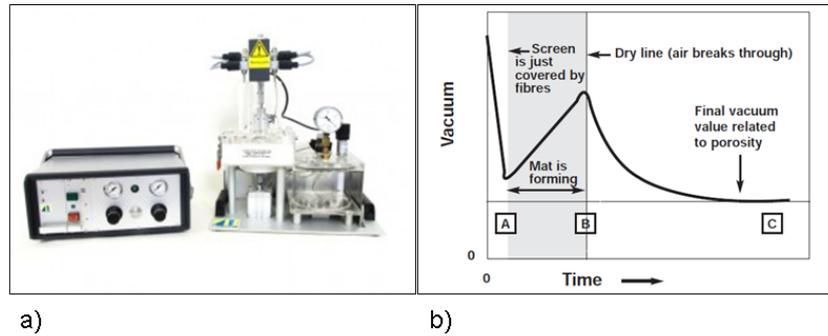
**Figure 3.2** The Dynamic Drainage Analyser as well as the result. a) The measuring device. In principle this equipment is a modification of the earlier developed DDJ as presented in 3.1. It consists of a cylindrical jar where the sample is collected, dosing devices for chemicals, an impeller for agitation, a changeable screen, a filtrate chamber and a vacuum device to support drainage, the vacuum level is detected by a transmitter [Wirth et al., 1999].
