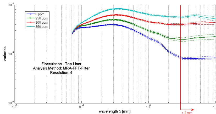
**Figure 6.5** The influence of a single polymer retention system on flocculation. The sample without dosage of the polymer clearly show the lowest flocculation. By increasing the concentration of the polymer the flocculation increases too.
