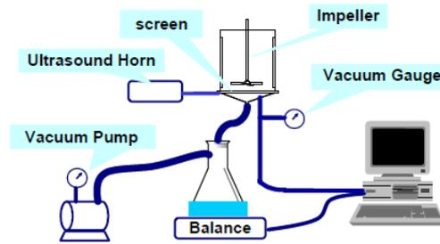
**Figure 3.6** This measuring device represents a modification of the Dynamic Drainage Jar. The principle constituents of this device are the drainage chamber equipped with an impeller, the filtration chamber, the balance and the vacuum pump. The special equipment of this device is an ultrasonic horn connected to the wire frame. The ultrasound energy produces additional effects like turbulences and acoustic forces influencing drainage [Ju et al., 2011].
