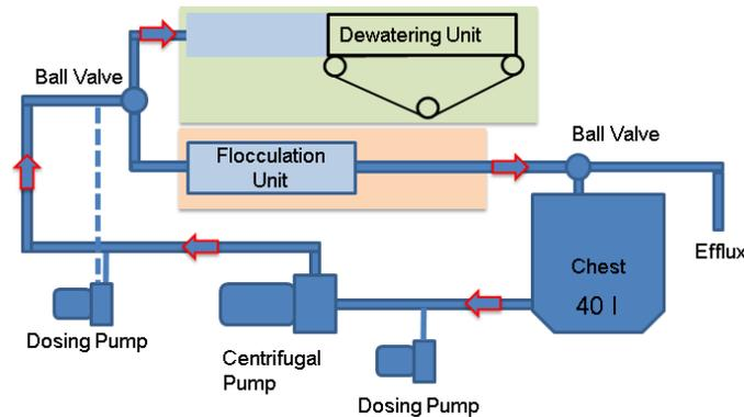
**Figure 4.1** A schematic illustration of the novel laboratory device. The device consists of a pulp chest, a centrifugal pump, two dosing pumps and three dosing points. The device is divided into two units, the flocculation unit with a transparent observation channel and the dewatering unit including a headbox and a fourdrinier former section.
