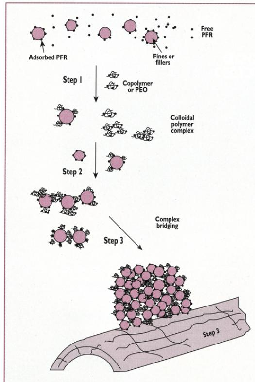
**Figure 2.4** The functional principle of network flocculation. In the shown system a phenolic formaldehyde resin (PFR) and a polyethylene oxide (PEO) is used. This system is similar to the dual polymer flocculation and occurs for dispersed components like fillers and fines [Xiao et al., 1996]
