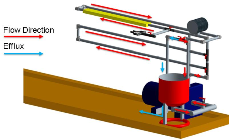
**Figure 4.4** The flow direction in the loop setup. Starting from the pulp chest the suspension passes the centrifugal pump, the loop extension as well as the flow meter, after the ball valve at the end of the loop back to the chest. The red bars show the circulation of the suspension in the flow loop, the blue bars show the flow if the suspension leaves the closed cycles.
