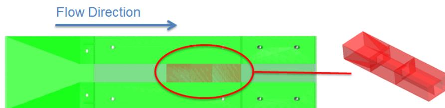
**Figure 4.16** The diffuser is made of transparent polycarbonate. By means of the diffuser with an entire length of 260 mm the fibrous suspension is accelerated. To achieve flow velocities comparable to a real headbox a step diffuser (red block) can be integrated. At the outlet of the diffuser the cross section changes abruptly from 25 x 15 mm up to a cross section of 35 x 25 mm and turbulences are generated.
