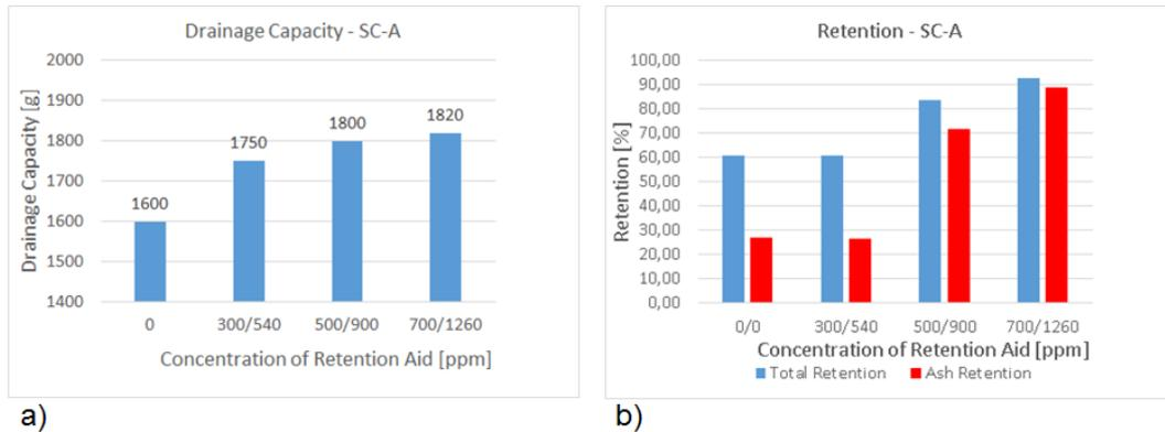
**Figure 6.4** a) Evaluation of drainage capacity. Drainage is improved up to a concentration of 500 ppm PAM and 900 ppm PVAM and remain roughly static.
