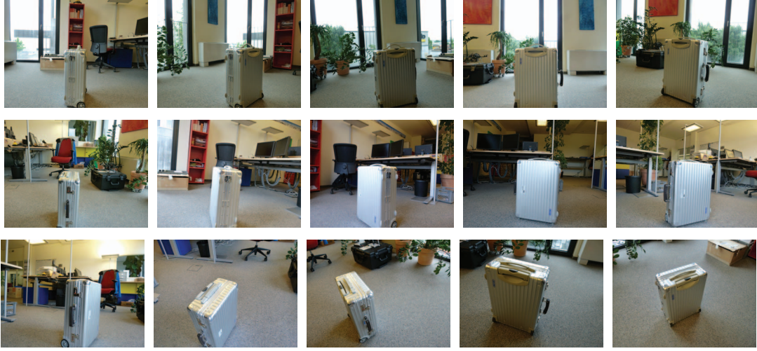
Figure 1.7: Typical dataset for the reconstruction of the suitcase acquired by a non-expert user. The floor is very repetitive and the texture of the suitcase creates only a few feature points. Furthermore, the angles between the images are very large. State-of-the-art SfM pipelines are not able to successfully reconstruct the scene using the input images.
