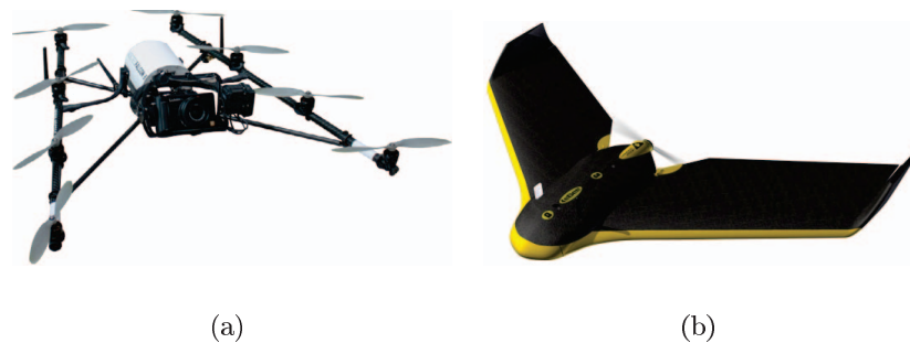
Figure 1.3: Two different Micro Aerial Vehicles. (a) Asctec Falcon 8 octo-copter equipped with a 16 Mpx still image camera. The flight time is around 20 minutes and the operation height varies between 3 m and 150 m above ground level. (b) The Ebee MAV manufactured by Sensefly is a fixed-wing MAV equipped with a 12 Mpx still image camera. After the definition of a flight plan, it operates up to 45 minutes autonomously. The camera is mounted such that nadir images are collected. Its operation height is between 70 m and 300 m.
