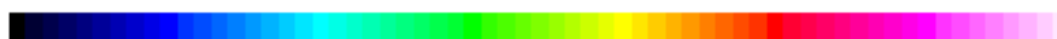
Figure 4.3-XLIX: Colour coding used for all elemental maps; increasing concentrations are represented by the colour line starting from black illustrating no content over blue, green, yellow, red and violet up to white for the highest content
