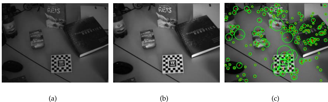
Figure 4.18: Image acquisition and processing. (a) Image grabbed from the camera device. (b) After distortion correction using the parameters from an offline calibration process. (c) Extracted SIFT keypoints (red) and their descriptors (green), which are used for data association and map point generation.
