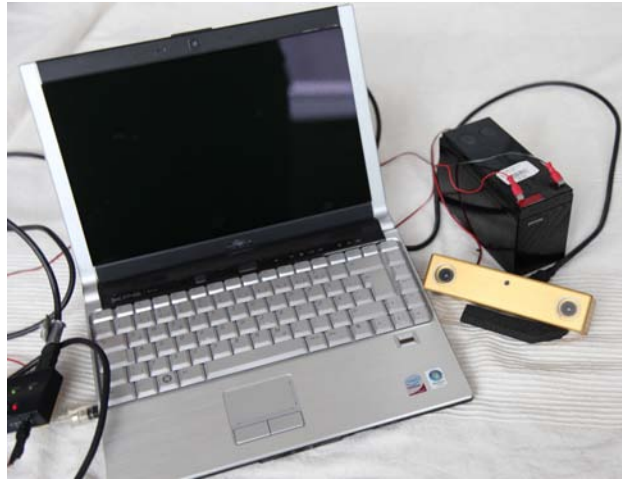
Figure 6.3: Hardware setup. The camera is attached through Firewire to a consumer laptop. For electric power supply we used a 12V lead-acid battery.
