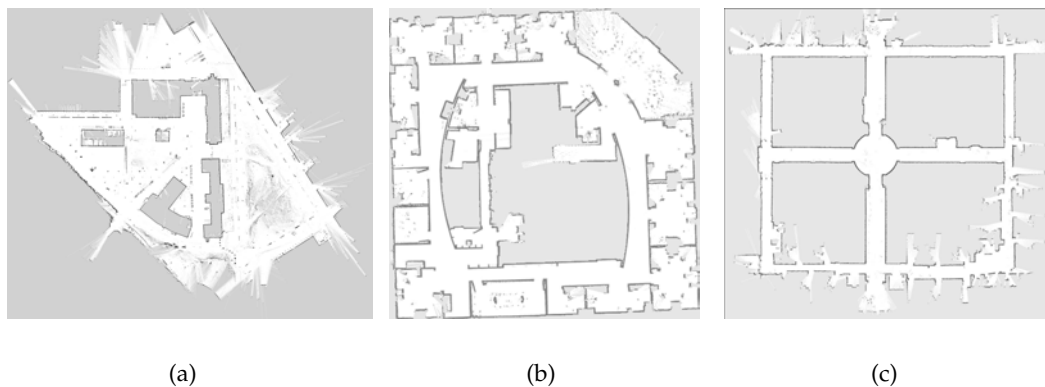
Figure 6.1: Estimated maps of the Radish dataset repository all consisting of laser and odometry data. (a) Freiburg Campus dataset (courtesy of [125]). (b) Intel Research Lab dataset (courtesy of [47]). (c) ACES Texas dataset (courtesy of [44]).
