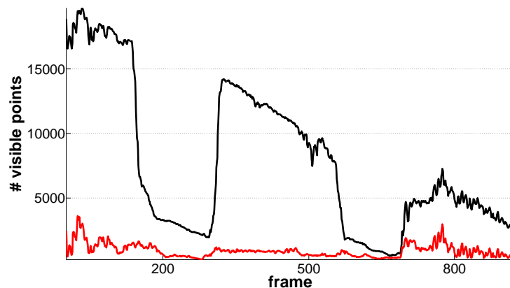
Figure 6.12: Moving camera - moving scene: Data association evaluation. Putative matching candidates per frame with (red) and without (black) using visibility information for the run highlighted green in Figure 6.18 are compared. We reduced the number of visible map points from 7753 to 902 per frame on average.
