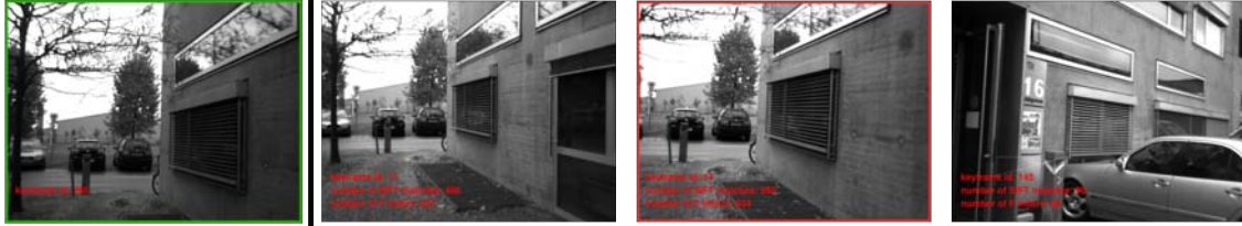
Figure 4.21: Geometric verification of the loop closure candidates for the query image framed green. Wrong voctree responses are filtered out through descriptor matching followed by fundamental matrix estimation. The keyframe producing the most RANSAC inliers is reported to be the loop closing frame \mathbf{P}_1 (framed red).
