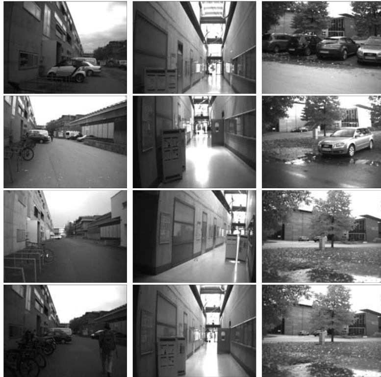
Figure 1.4: Challenging scenarios when performing visual SLAM. Short-term changes such as moving persons or driving cars lead to distorted sensor readings. Different lighting conditions, moved furniture or various weather situations pose a challenge for every camera-only SLAM algorithm.
