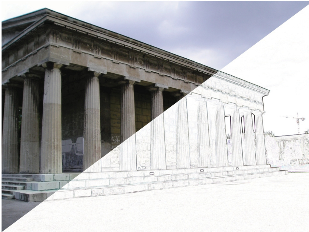
Figure 1.2: A Laplace filter eliminates same-color regions and highlights edges. Assuming that a point on an edge will have corresponding points that are also located on edges, a Laplace filter reduces the amount of input data to solve the corresponding point problem and to find a stable solution.
