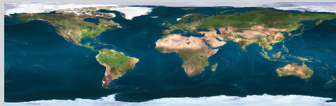
Figure 3.13: This ARCHIMEDEAN map of the earth preserves areas; i.e. if two regions have the same size, then their images also have the same size.
