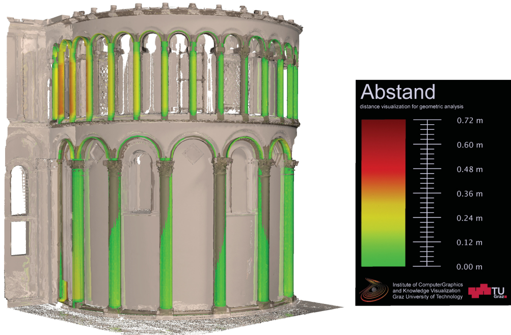
Figure 5.13: A generative model with nine parameters is fitted to the laser scan of the Duomo of Pisa. The algorithm detects two instances of the shape template and determines the parameters which describe the given geometry best. These characteristics (column height, etc.) are high-level parameters and valuable information which are needed in the context of digital libraries in order to index a model repository.
