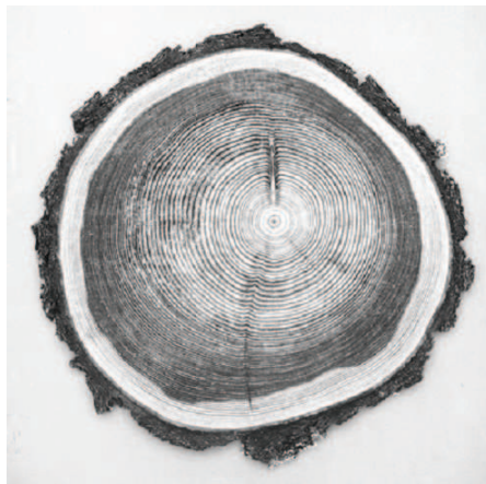
Figure 1.1.: Transverse cross section of a timber with clearly visible annual rings, adopted from (Gullichsen and Paulapuro 1999)
