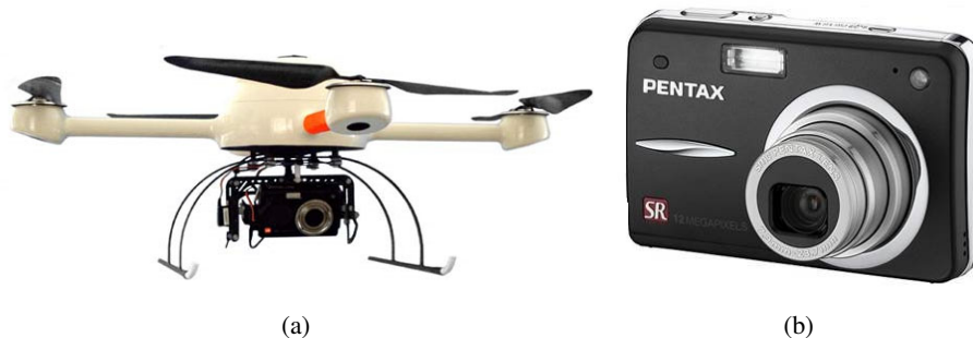
Figure 3.19: (a) Micro-drone md4-200 with attached PENTAX Optio A40 (b).
