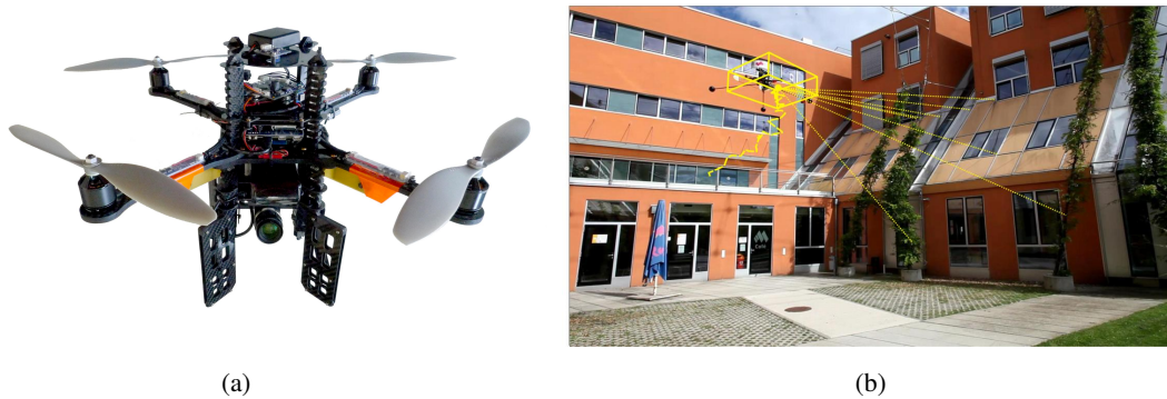
Figure 6.5: (a) Pelican quad-rotor MAV from Ascending Technologies equipped with a single, wide angle camera used for localization. (b) Localization result of our proposed algorithm with respect to the reconstructed scene.
