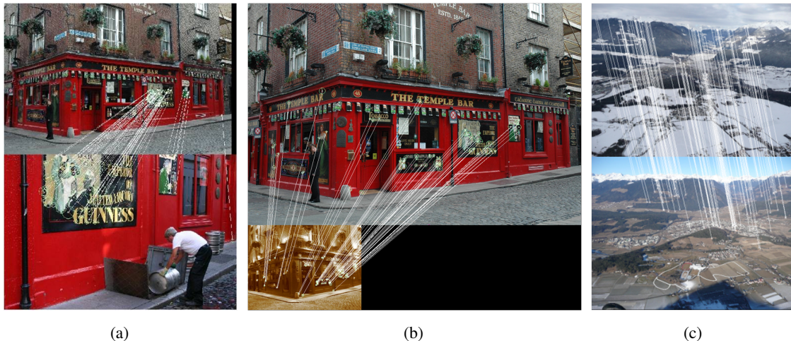
Figure 2.5: Natural feature matching results based on the Scale Invariant Feature Transform (SIFT) for challenging image pairs, (a) large scale and viewpoint changes, (b) illumination changes (e.g. day, night) and (c) large scene variations (e.g. summer-winter scene). Lines indicate corresponding points that satisfy the epipolar geometry. Even though the distortion of the images is significant a large number of correct correspondences is obtained. This would not be possible using conventional feature detectors like Harris corners and local intensity patches.
