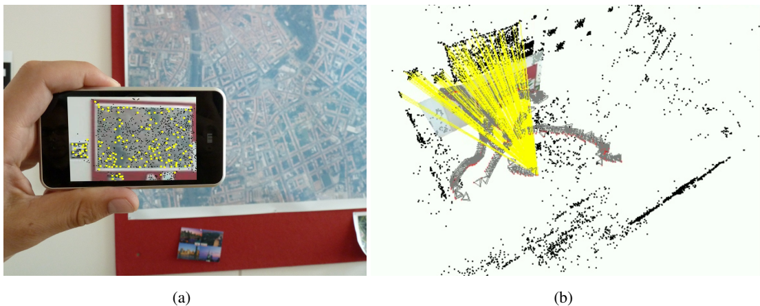
Figure 6.14: Camera pose tracking using the Meizu M8 smart-phone in an indoor environment. Yellow lines depict inlier of 3D-2D point correspondences.
