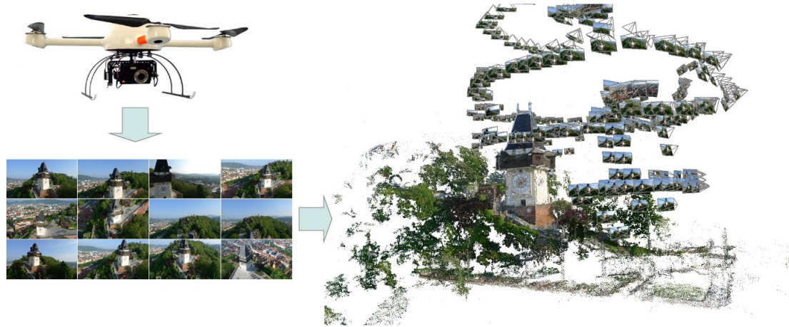
Figure 1.6: Micro-drone md4-200 with attached PENTAX Optio A40 and reconstruction of the clocktower of Graz from 420 images.
