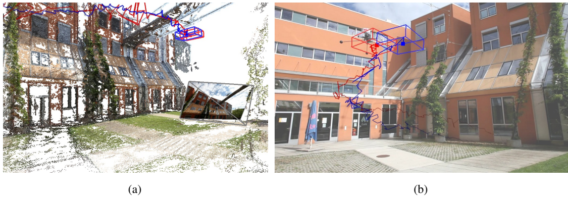
Figure 6.12: Visual comparison of the localization results via registered ground truth video stream. (a) Oblique view of registered ground truth showing the current camera frame and MAV positions (path and bounding box) estimated by our localization approach (red) and the aligned PTAM result (blue). (b) Back-projected bounding box from the observer's point of view.
