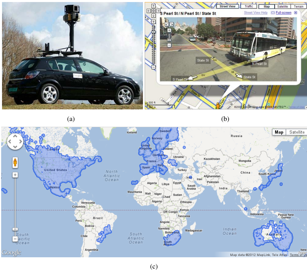
Figure 1.4: (a) Google Street View car with mounted 360° camera system for large scale terrestrial mapping and (b) Street Maps Sphere viewer. (c) Current world wide coverage of street view data (Januray 2012).
