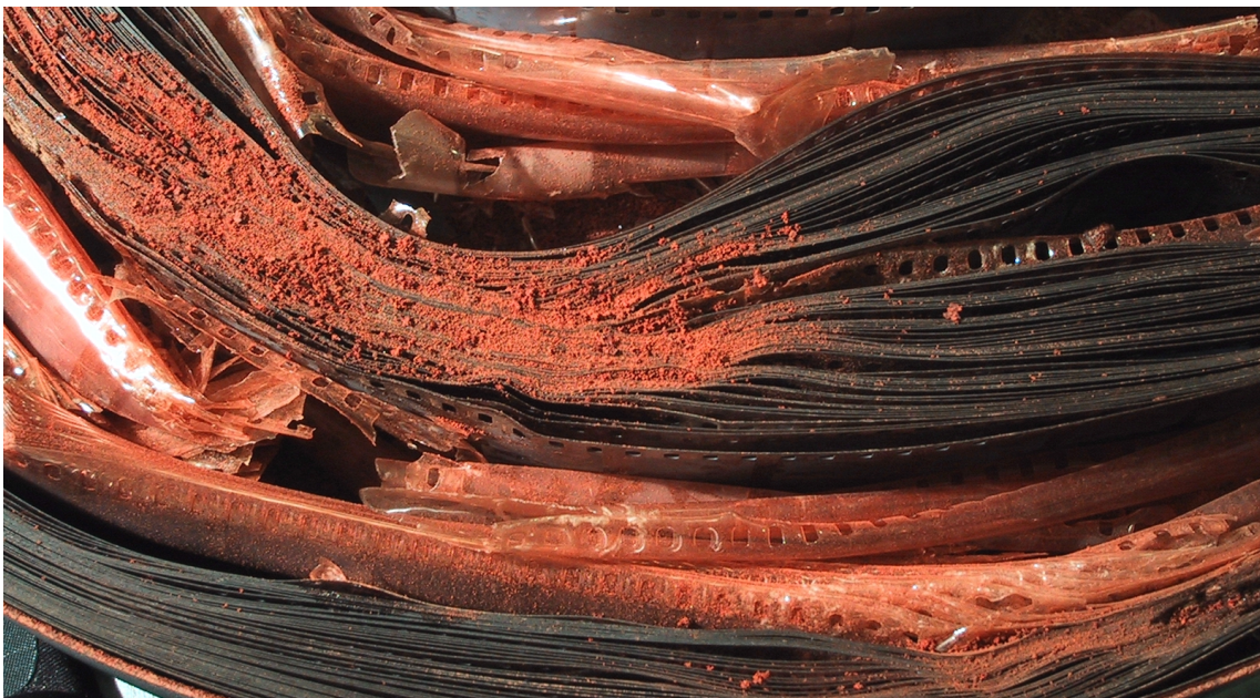
Figure 2.2.: Combination of nitrate and triacetate film. In this case the more modern triacetate film decomposes (vinegar syndrome) and then degrades the nitrate film too. © kino-eye, www.flickr.com
