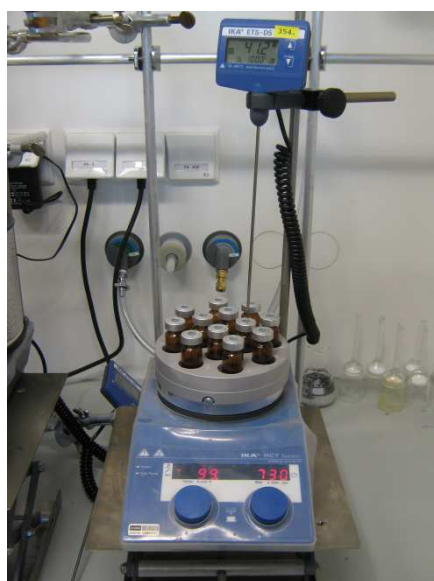
Fig. 85: Picture of the apparatus used for hydrazone synthesis
