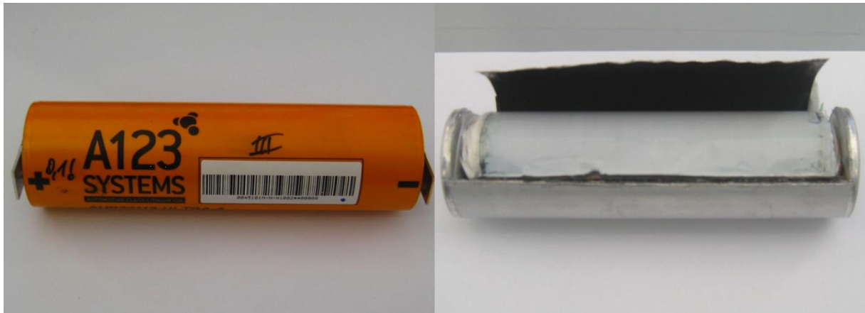
Figure 29: Image of the investigated cylindrical 3.6 Ah- cells.
