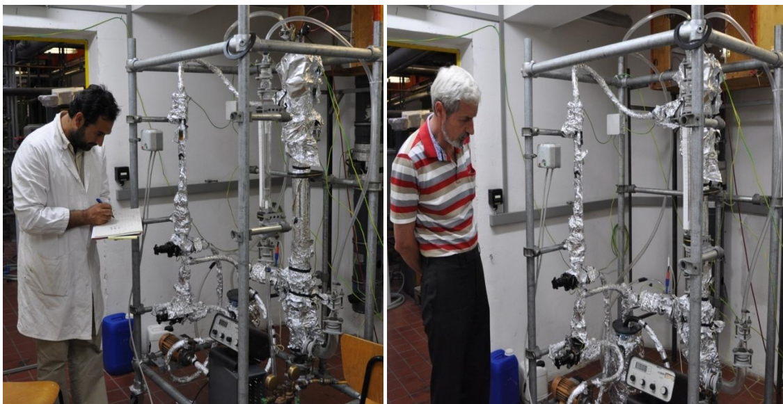
Figure 21: wet electrostatic precipitator in operation for actinometric measurements; the equipment was properly wrapped in aluminium foil. Prof. Dr. M. Siebenhofer is inspecting the operation of WESP.
