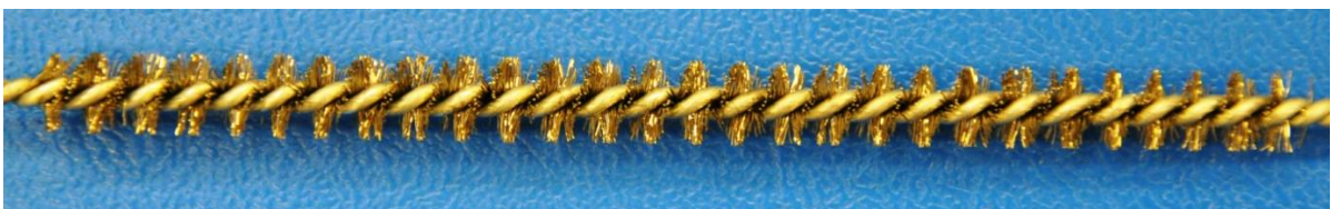
Figure 13: Brush type discharge electrode (stainless steel 8 mm diameter)
