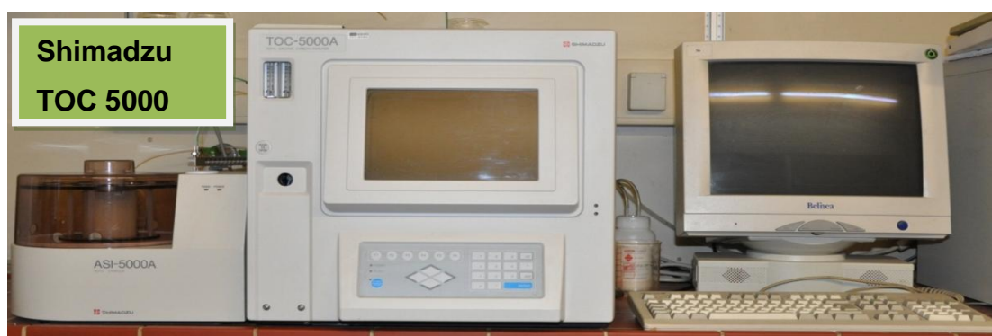
Figure 23 TOC analyzer used to measure concentration of organic carbon in terms of TOC in treated samples.
