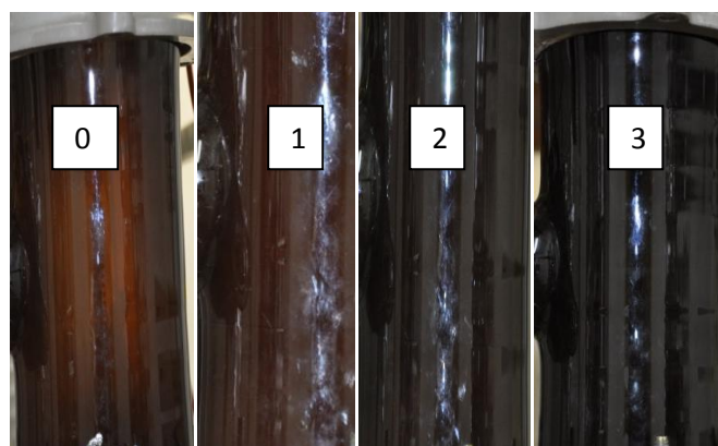
Figure 81: Colour change of industrial waste water containing phenol solution from light brown to black-brown color during treatment in the wet tube type electrostatic precipitator. Image also shows falling film and corona discharge from discharge electrodes. Samples were collected after every 4 h.
