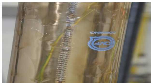
Figure 18: Complete film developed during the operation of WESP ( water is circulated from top)
