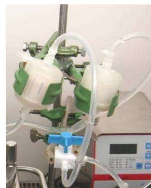
Figure 3.14 – Pall™ Mini-Kleenpak sterile filters with three-way stop cock
