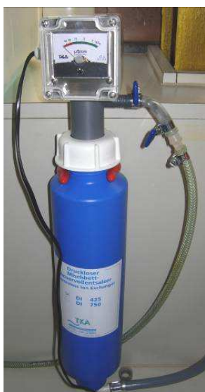
Figure 3.9 – Pressure less ion exchanger DI 425
