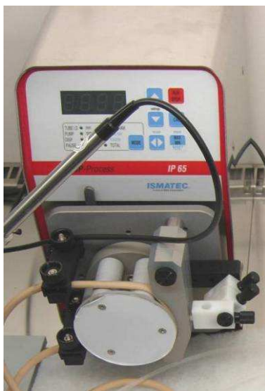
Figure 3.6 – Ismatec™ MCP-Process IP 65 peristaltic pump
