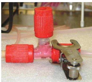
Figure 3.15 – Bubble trap working in a running experiment
