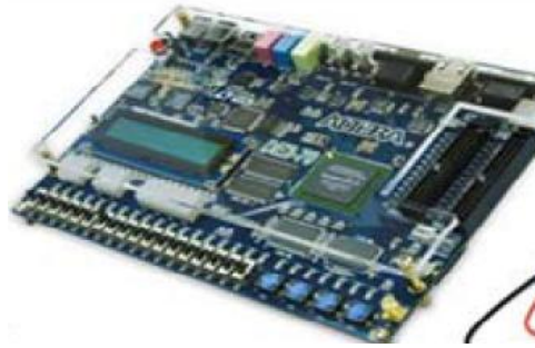
Fig. 4.1: DE2-70 Altera Board
