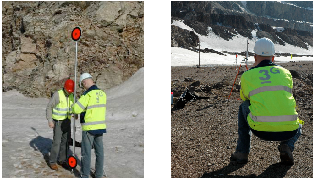
Figure 9: Installing a range pole in front of a rock face (left). Determining the azimuth of a reference line for North correction. Note the two marking elements (right).
