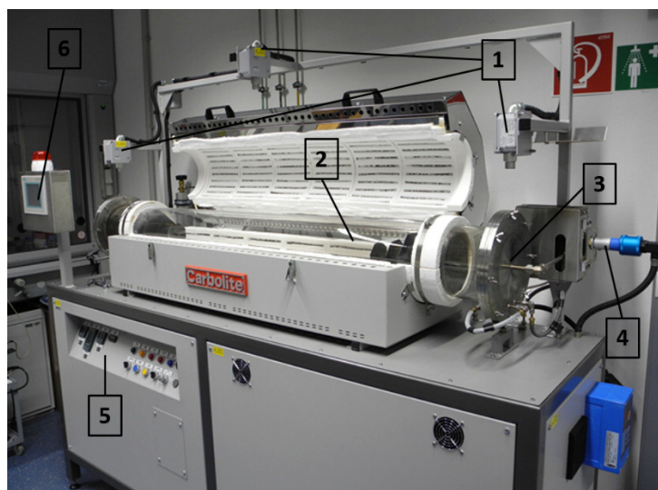
Figure 124: Set up of the HZS 12/200/1200; 1) Hydrogen leak detector, 2) Quartz tube with radiation shields on both sides, 3) water cooled flanges, 4) Pilot safety burner, 5) Temperature/Alarm control, 6) Touchscreen control panel
