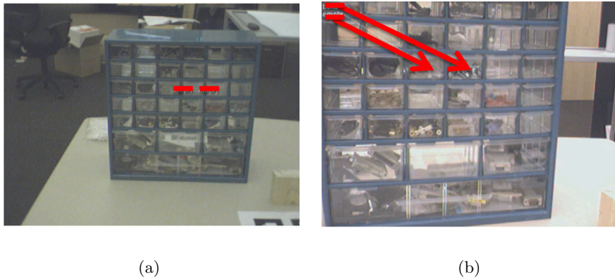
Figure 2.6: Ambiguities when using internal labels. (a) Without registration error the labels (highlighted red) would fit into the projected area of the drawers. However, a small registration error creates ambiguities. The labels cannot be associated with certain drawers anymore. (b) The leader lines of external labels are more tolerant to registration errors and can resolve such ambiguities (Images adapted from Coelho et al. [28]).
