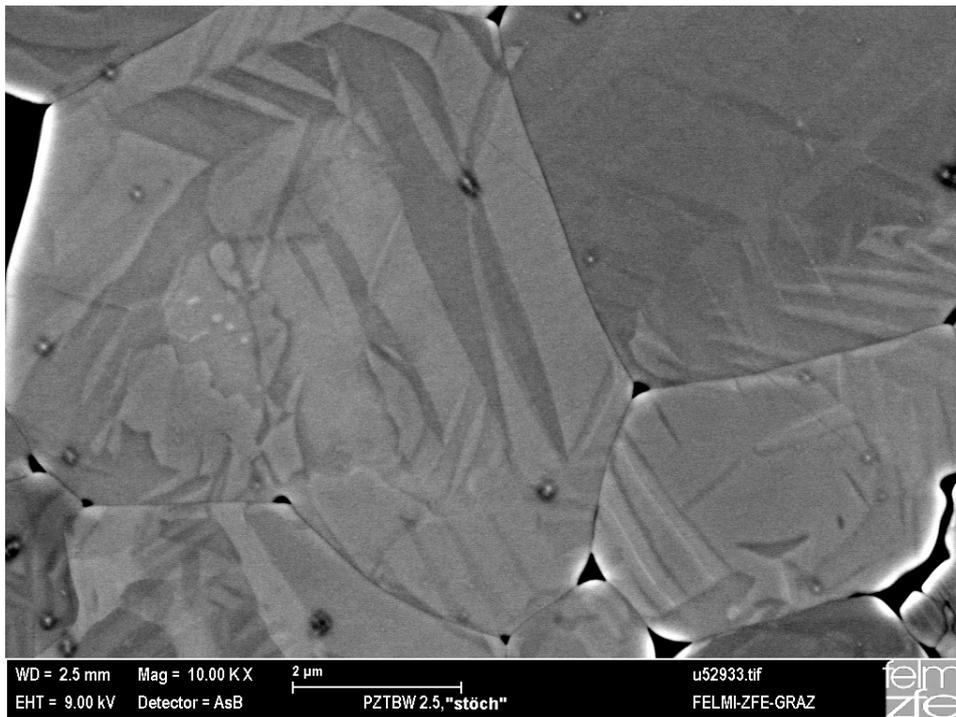
Figure 8: Ferroelectric domains in PZT made visible through channeling contrast imaging
