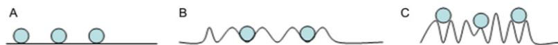
Fig. 1. Impact of surface roughness on interparticle interactions. Depending on the shade of the surface roughness meaning the distance between the roughness peaks and valleys the contact area can be altered and thus interparticle interactions.
