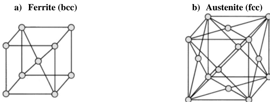
Figure 10. Crystallographic structures of pure iron for a) ferrite and for b) austenite.
