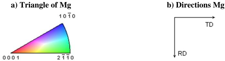
Figure 28. a) IPF triangle showing the colour coded orientation and b) RD and TD directions.
