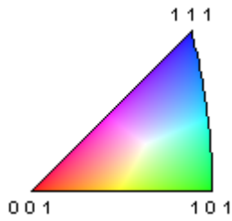
Figure 77. Unit triangle of ferrite for the EBSD orientation maps.
