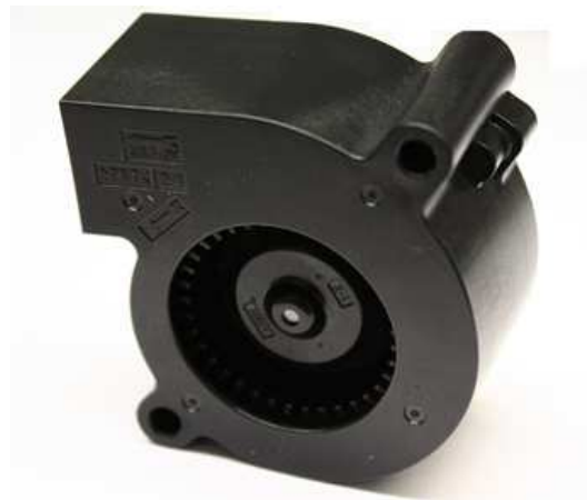
(b) External view of developed, integrated electric drive.
