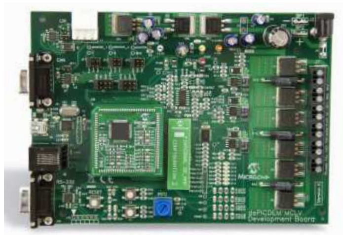
(a) dsPICDEM MLCV-2 development board.
