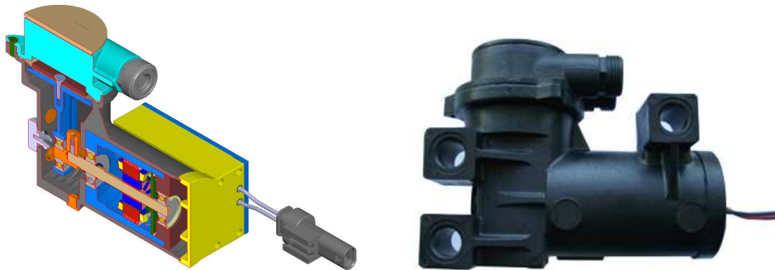
(a) Cross-sectional drawing of a pump with (b) External view of developed, integrated electric drive.
