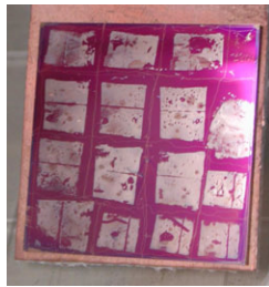
Figure 3.43: Sample with several \mu TP -OFETs fixed on a single-sided copper board.
