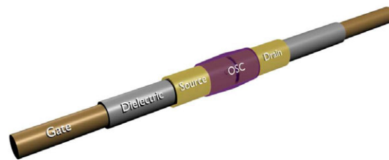
Figure 3.48: WireOFET architecture with copper wire as gate electrode and insulation layer as gate dielectric; OSC... organic semiconductor.
