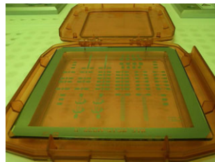
Figure 3.4: Typical 4" x 4" photolithography shadow mask (chrome on quartz glass), divided in 1" x 1" sectors with various target structures; critical dimension: 2 \mu\text{m} \pm 0.1 \mu\text{m} , no defects/ \text{cm}^2 > 2 \mu\text{m} .
