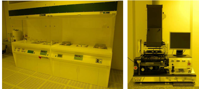
Figure 3.1: Photolithography equipment implemented in an ISO class 6 cleanroom environment, including a custom-made wet bench (left) and an EVG 620 top-side mask aligner (right).
