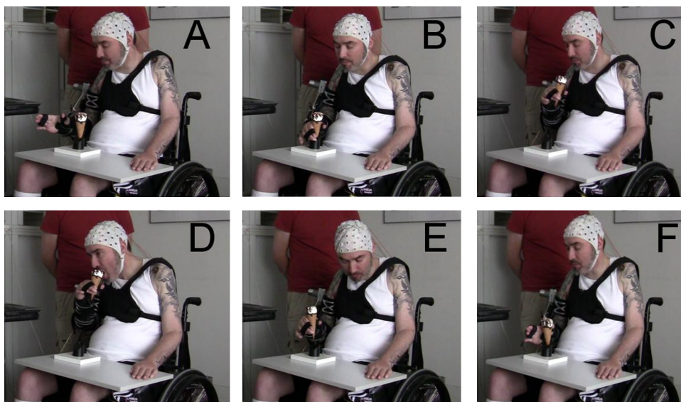
Fig. 7. Sequence of pictures showing the subject eating an ice cream cone. The user starts in the hand control mode, lifts his left shoulder to open the right hand to grasp the ice cream cone (A). After successfully grasping the ice cream cone (B), the user emits a BCI command to switch from hand control to elbow control and lifts his shoulder to flex his elbow (C). Now, the user licks the ice cream (D). Finally, the user lowers his left shoulder to extend the elbow (E) puts the cone back in its original place and switches back to hand mode to release the cone (F).
