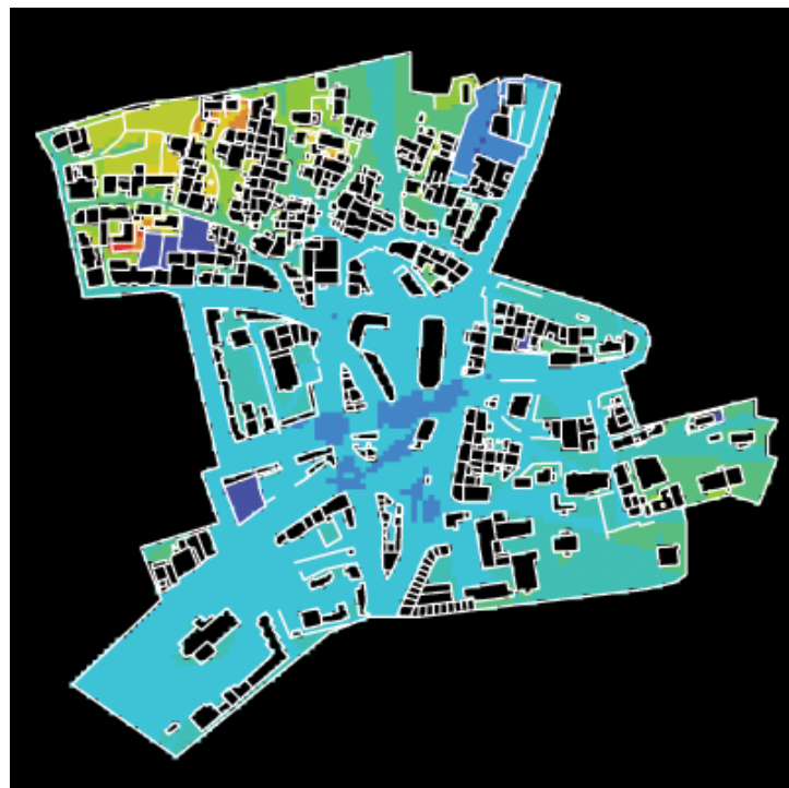
Figure 7.24: Mean depth values of the original and transformed public space network (note that the red color means the highest mean depth value and lowest integration spot, and the blue color means the lowest mean depth value or highest integration spot)
