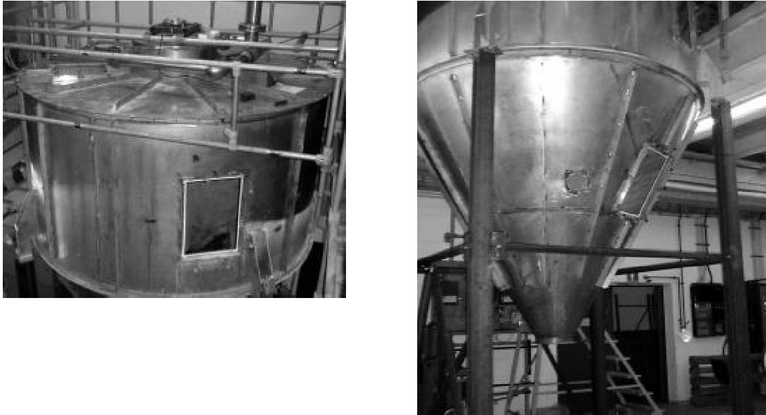
Figure 5. Images of the pilot scale spray dryer (proprietary construction, group Prof. Walzel, Dortmund University of Technology)
