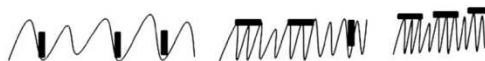
Fig. 11. Influence of surface roughness on interparticle forces between carrier and micronized active. Depending on the size scale of the surface roughness and the particle size of the active, the contact area and hence interparticle forces may be modified.
