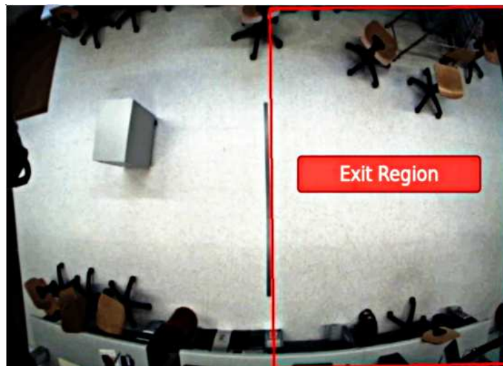
Figure 6.11: EAS scenario: Camera view with highlighted exit region . The camera view shows a considerable distortion due to the use of a wide angle lens which is required to provide an adequate field of view.
