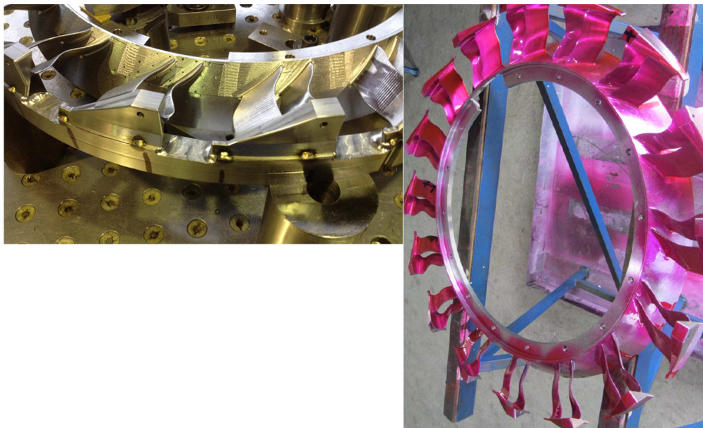
FIGURE 3.10: Manufacturing and integrity checkup of the splitter bladed ring
