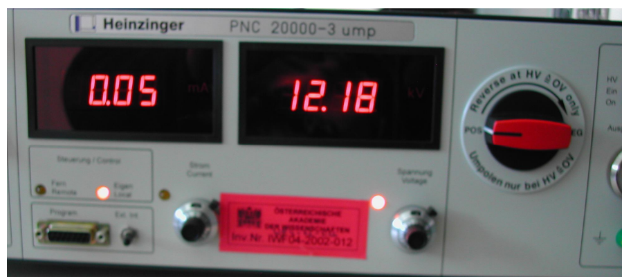
Figure 4-15: High voltage power supply unit (HV-PSU)
