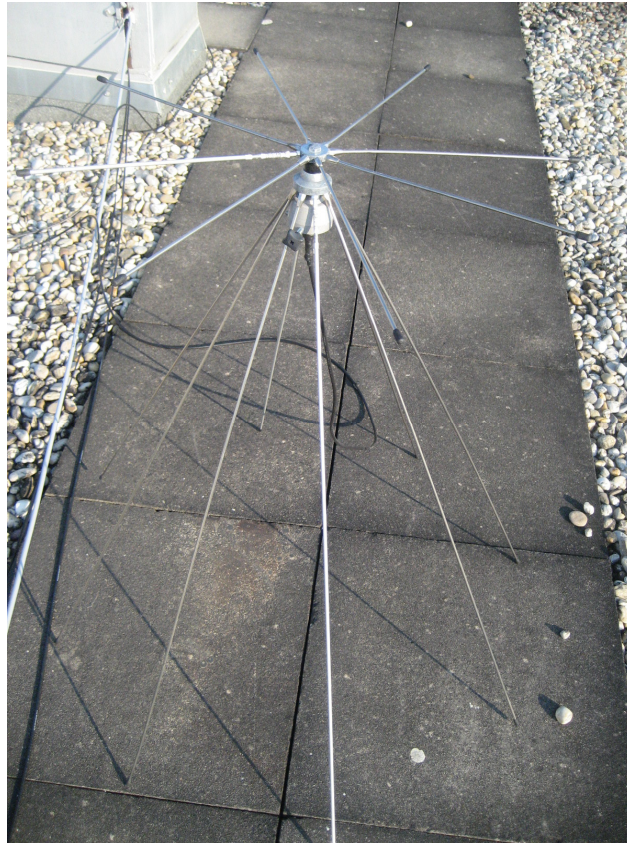
Figure 4-21: The broadband discone antenna used for natural lightning measurements. The antenna was put on the roof of the TU Graz building for better reception and to avoid interferences within the campus.
