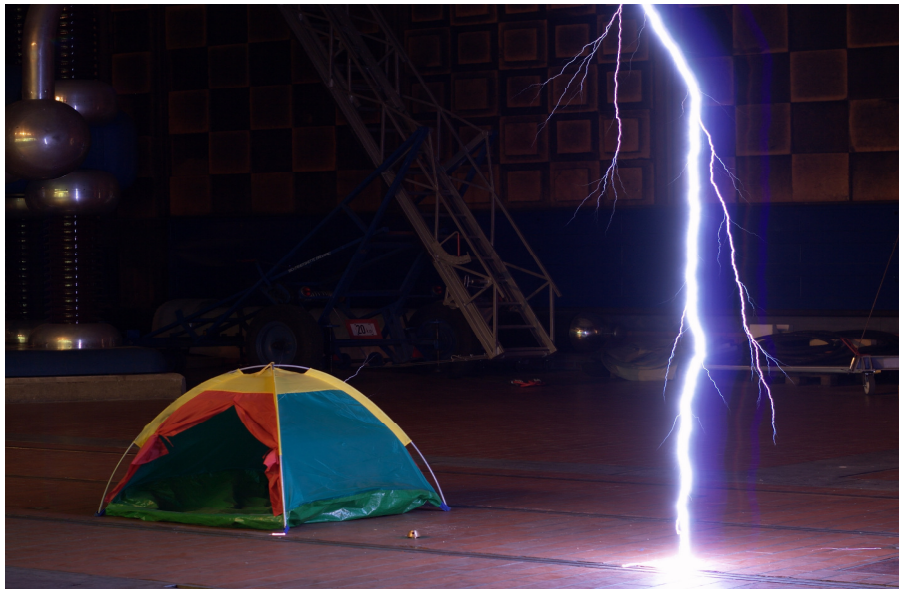
Figure 4-8: Lightning event occurs near the object due to slight movement of the electrode.
