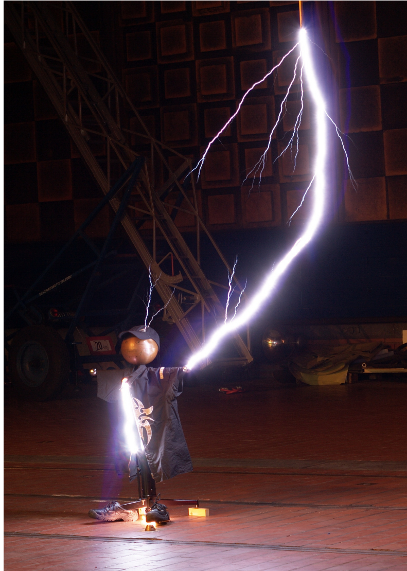
Figure 4-3: Lightning event occurrence on a model. Also branched lightning (to ground and air) was observed.
