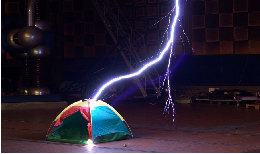
Figure 4-7: The basic structure of the tent serves as a model for the Faraday cage. There can be arcing if some metal is present inside the tent (no lightning safety)
